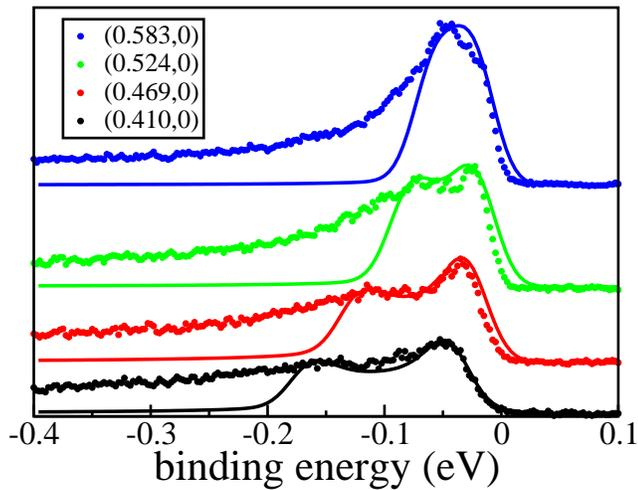
Fig. 1 – Selected ARPES data (dots) from Ref. [11] and the fitted spectral intensities (solid lines) within the Luttinger liquid phenomenology for different  $|\mathbf{k}|$  vectors along  $\Gamma - M$  direction of the Brillouin zone. The  $|\mathbf{k}|$  vector values are in  $\text{\AA}^{-1}$  units.
