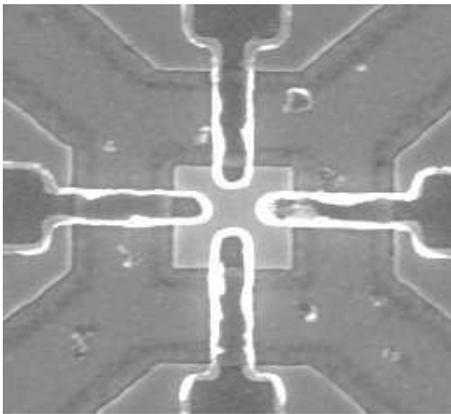
FIG. 2: Quantum dot (central square of dimensions 500 nm  $\times$  500 nm) fabricated in a high-mobility InAs/AlSb heterostructure and contacted by four superconducting Nb electrodes. Device made by A. T. Filip, Groningen University (unpublished figure).
