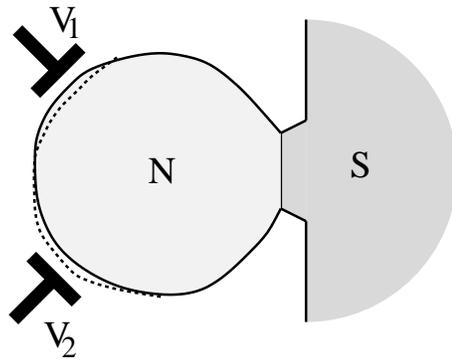
FIG. 5: A quantum dot (N) connected to a superconductor (S). The voltages on the gates  $V_1$  and  $V_2$  change the shape of the dot. Different values of the applied voltages create different samples within the same ensemble. From Ref. [34].
