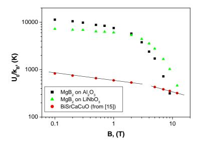
Fig.5. Dependence of the activation energy  $U_0/k_B$  on magnetic field for the investigated samples (solid quadrates, 400 nm thick MgB<sub>2</sub> film deposited on sapphire; solid triangles, 5µm thick film deposited on LiNbO<sub>3</sub>). For comparison, the weak power-law dependence  $U_0 \sim B^{-n}$ , n = 1/6 and n = 1/3 for two linear parts of the  $U_0(B)$  dependence, for a high- $T_c$  superconductor (solid circles, data for Bi-Sr-Ca-Cu-O sample taken from [15]) is given.
