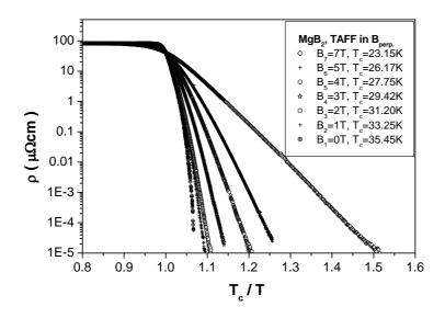
Fig. 4 Arrhenius plot of  $\rho(T) \mid_{B=const}$  for the sample, presented in Fig.3. From the slope of the linear parts of the curves the values of the activation energy  $U_0$  are obtained. The Arrhenius plot in Fig. 4 presents the data of Fig. 3 as  $ln(\rho)$  against  $(T_c/T)$ .
