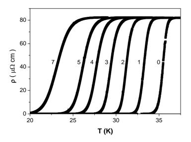
Fig. 3 Resistive transitions  $\rho(T)$  for a 400 nm thick MgB<sub>2</sub> film at different values of the magnetic field perpendicular to the film plane: curves 0 to 7 correspond to B = 0, 1, 2, 3, 4, 5, 7 Tesla.
