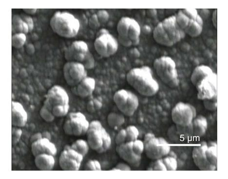
Fig.1 Electron microscope (SEM) image of  $5\mu$ m thick MgB<sub>2</sub> film on a LiNbO<sub>3</sub> substrate (scan size 20  $\mu$ m x 15  $\mu$ m, 5KV); a rough island covered surface with a wide distribution of island size up to 5  $\mu$ m were imaged.
