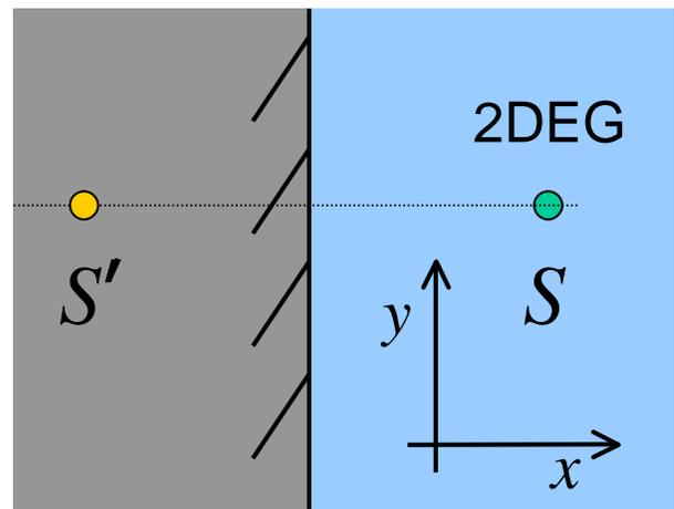
FIG. 1: Schematic of the system: 2DEG occupies half-plane  $x > 0$ . The influence of the boundary located at  $x = 0$  on the electron space motion is taken into account by introducing the mirror source  $S'$ .
