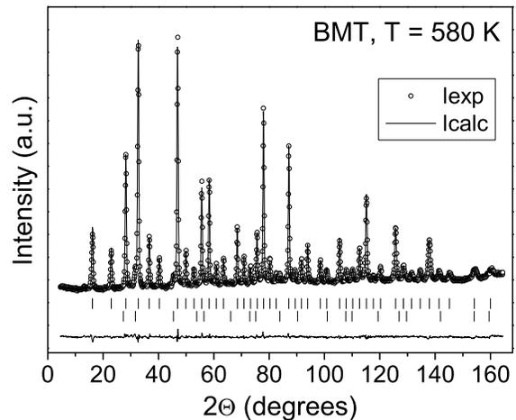
FIG. 1: Neutron powder diffraction pattern of BMT collected at  $T = 580 \text{ K}$ . Observed data points, calculated profile and difference curve are shown. The two rows of ticks correspond to the calculated positions of diffraction peaks for BMT (upper) and MgO impurity (3%).
