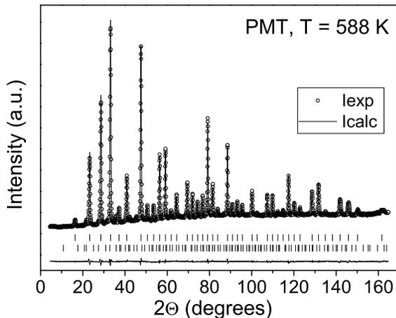
FIG. 2: Neutron powder diffraction pattern of PMT collected at  $T = 588$  K. Observed data points, calculated profile and difference curve are shown. The two rows of ticks correspond to the calculated positions of diffraction peaks for perovskite PMT (upper) and pyrochlore impurity (5 %).
