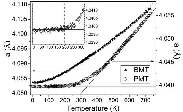
FIG. 4: Temperature dependence of the lattice parameters of PMT and BMT. The solid lines show the results of linear extrapolation for the  $a(T)$  dependence of PMT. The dashed line shows the polynomial fit of  $a(T)$  for BMT. The insert shows the dependence of the lattice parameter of PMT in the region of temperatures around  $T \sim 180$  K. Invar-like behaviour of PMT for  $T < 180$  K is obvious.
