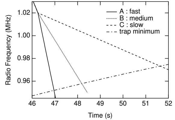
FIG. 1: Time dependence of radio-frequency during the final stage of evaporative cooling used in this experiment. The origin of the time scale represents the starting point of the evaporative cooling. Frequency changing rate for each RF sweep is 96.8 kHz/s (A: fast), 32.3 kHz/s (B: medium), and 8.7 kHz/s (C: slow), respectively. The drift of the trap minimum is 4.6 kHz/s.
