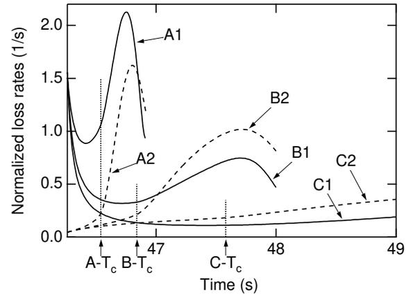
FIG. 3: Loss rates for the three kinds of RF sweep normalized by the total number of trapped atoms at each time. A, B, and C represent the fast, medium, and slow RF sweep, respectively. The solid curves (A1, B1, and C1) represent the loss rates caused by evaporation and the dashed ones (A2, B2, and C2) represent those caused by three-body recombination, respectively.  $A-T_c$ ,  $B-T_c$ , and  $C-T_c$  represent the BEC transition point for each RF sweep.
