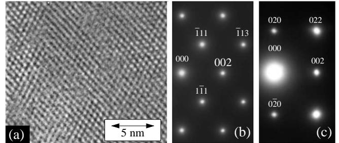
FIG. 2: (a) High resolution image of [110] $\{\text{FeC}_2\text{S}_4$ . (b) SAED pattern of [110] and (c) [100] oriented samples.
