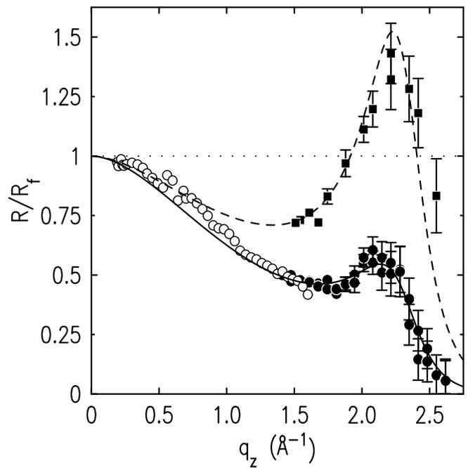
FIG. 2: Specular x-ray reflectivity for liquid Indium at 170 °C taken with vertical detector resolutions of  $0.06$  Å<sup>-1</sup> (scintillation detector; open circles: X22B, closed circles: X25) and  $0.32$  Å<sup>-1</sup> (PSD in single channel mode; squares: X25). The reflectivity is normalized to the Fresnel reflectivity  $R_f$  of a flat In surface. Solid lines are fits as described in the text. Data from X22B was not incorporated in any fits.
