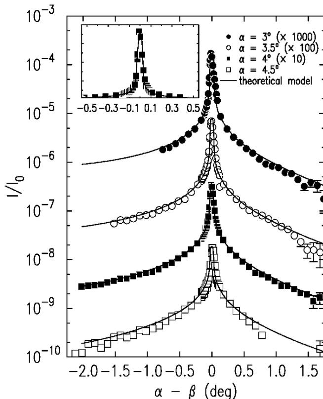
FIG. 3: Diffuse scattering as a function of scattering angle  $\beta$  for different fixed incoming angles  $\alpha$ . Solid lines: Diffuse scattering calculated from the experimentally determined structure factor with no further adjustable parameters. Inset: linear plot emphasizing the fit near the specular peak for  $\alpha = 4.5^\circ$
