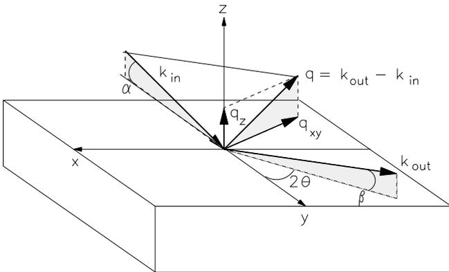
FIG. 1: Sketch of the geometry of x-ray scattering from the liquid surface with  $\alpha$  and  $\beta$  denoting incoming and outgoing angle, the incoming and outgoing wavevector  $\vec{k}_{in}$  and  $\vec{k}_{out}$  respectively and the azimuthal angle  $2\theta$ . The momentum transfer  $\vec{q}$  has an in-plane component  $q_{xy}$  and a surface-normal component  $q_z$ .
