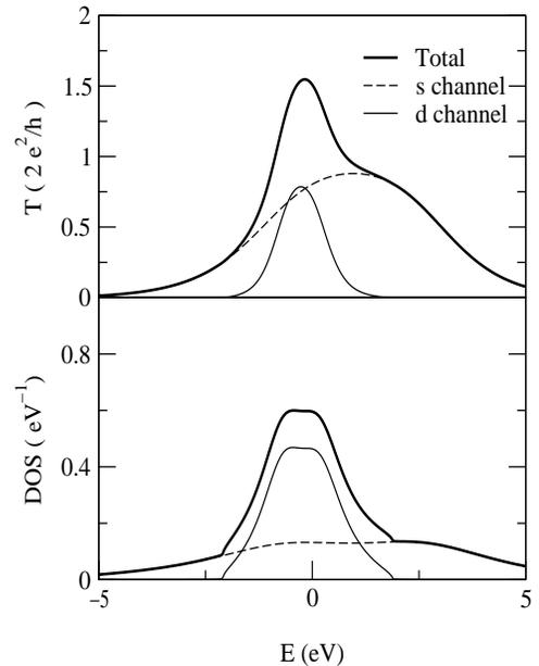
FIG. 2: Upper panel: transmission as a function of energy for the Pt<sub>2</sub> cluster. Total transmission (thick continuous line) and the contributions of the  $d$  (continuous line) and  $s$  (broken line) eigenchannels are shown. Lower panel: same for the density of states (DOS).
