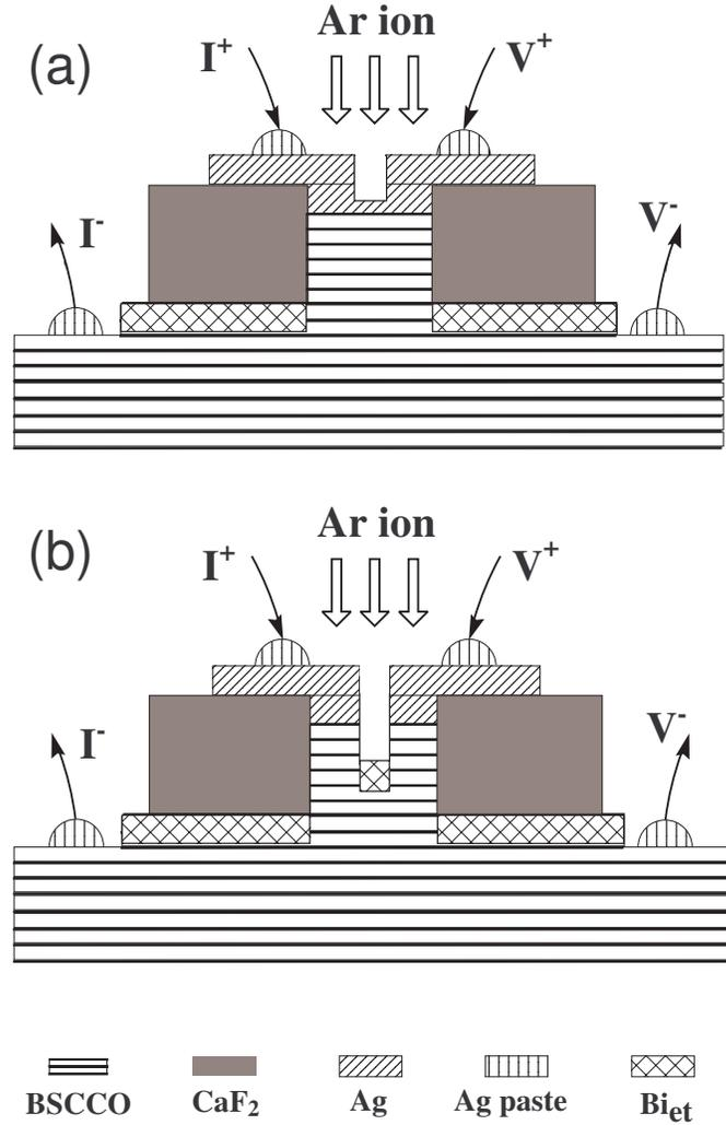
Fig. 1. Schematic view of IJJs of mesa structure. (a) when  $T_2 \leq (d_1 + d_2)/ER_{Ag}$ ; (b) when  $T_2 > (d_1 + d_2)/ER_{Ag}$ , where  $Bi_{et}$  represents the BSCCO layer damaged during the ion milling.
