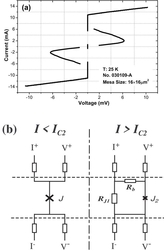
**Figure 6.** (a) Novel  $I - V$  curve of a single IJJ. The sizes of two top electrodes are both  $6 \times 16 \mu\text{m}^2$ ; (b) Equivalent circuits for the single IJJ at high bias current, where  $I_{c2}$  denotes the bias current at which the reentrance of super-current happens.
