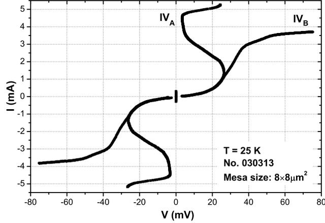
**Figure 5.**  $I$ - $V$  curves of a single IJJ when the bias current passes through different top electrodes. The sizes of the two top electrodes are  $1.5 \times 8\mu\text{m}^2$  ( $E_A$ ) and  $4.5 \times 8\mu\text{m}^2$  ( $E_B$ ) respectively.  $IV_i$  denotes that the bias current passes through top electrode  $E_i$  ( $i = A, B$ ).
