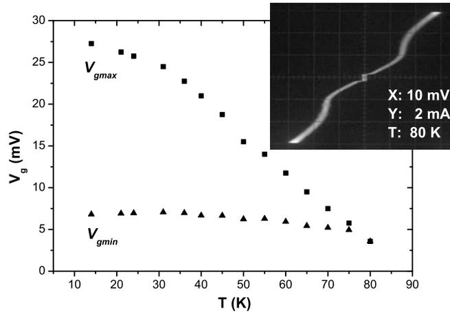
**Figure 4.** Temperature dependence of  $V_{gmax}$  and  $V_{gmin}$  for a 4-junction IJJs. The inset shows the  $I - V$  curve of the sample at  $T=80$  K
