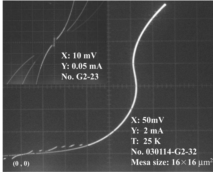
**Figure 3.** Three-terminal  $I - V$  curves of the sample sharing a top electrode for both current bias and voltage measurement. The inset shows the existence of a surface junction with a small critical current
