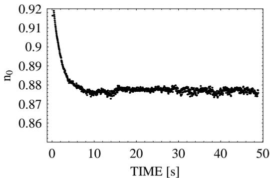
FIG. 1: Time-evolution of a zero momentum component  $|\alpha_{0,0,0}(t)|^2$ . A thermalization is clearly visible, as well as rapid fluctuations due to non-linear dynamics. The data have been obtained on a grid  $36 \times 36 \times 36$  and  $g = 18.515$ .
