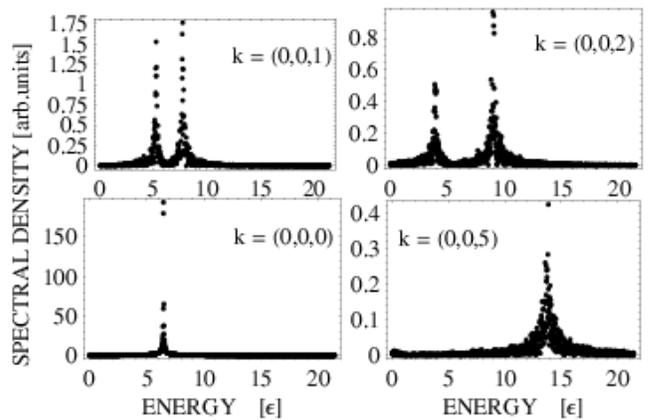
FIG. 2: Typical frequency spectra of plane-waves modes. The condensate mode (bottom-left) has a clearly defined energy  $\mu$ , while spectra of excited modes are broadened due to interactions. Note that one group of peaks is suppressed in  $(0, 0, 5)$  mode - the Bogoliubov transformation is practically a unit in this case. The parameters of the plot are:  $n_{grid} = 32$ ,  $g = 18.515$ ,  $n_0 = 86.2\%$ .
