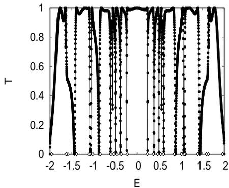
FIG. 1: Plot of the transmission coefficient,  $T$ , against the incident particle's energy,  $E$ , for a  $10 \times 10$  lattice with point to point contacts to the input and output chains. The diamonds ( $\diamond$ ) are the locations of the doubly degenerate eigenvalues of the isolated square lattice.
