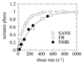
**Figure 19** : Percentage of the nematic phase induced by shearing obtained from flow birefringence [124], small-angle neutron scattering [124] and deuterium NMR [160]. Experiments are performed on a CTAB-D<sub>2</sub>O concentrated solution closed to I-N transition. The data from SANS and NMR are in good agreement.
