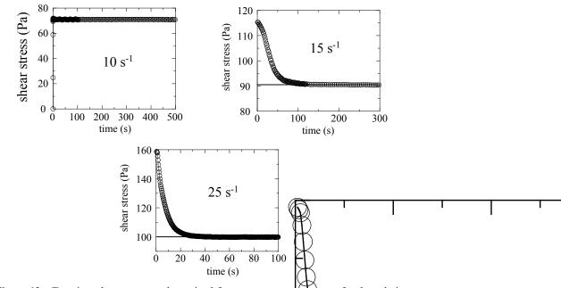
Figure 12 : Transient shear stress as determined from startup measurements for the solution shown in Fig. 11. Data are taken below and in the plateau region. The characteristic time of the initial stress decrease at 15 and 25 s<sup>-1</sup> is much larger than the Maxwell characteristic ( $\tau_R = 0.02$  s). The slow kinetics corresponds to the formation of shear bands.
