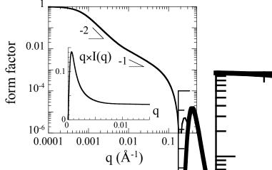
**Figure 3** : Scattering form factor of a wormlike micellar aggregate of total curv linear length L = 4  $\mu$ m, of persistence length b = 400 Å and of radius R<sub>C</sub> = 20 Å. Calculations were made using the Pedersen and Schurtenberger model [106]. The cross-over between the q<sup>-1</sup> and q<sup>-2</sup> regime is emphasized in the inset (Holtzer representation, q×I(q) *versus* q).
