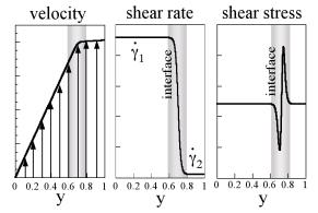
**Figure 24** : Velocity, shear rate and shear stress profiles calculated under the assumptions of shear banding and of non monotonic flow curve. In order to remove the spurious oscillations in the shear stress, a gradient term is needed (Eq. 17). This figure is taken from [224].
