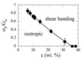
**Figure 21** : Concentration dependence of the reduced stress (closed circles) at the plateau for the CPCI-NaSal system [122]. At high concentrations, the values of  $\sigma_P/G_0$  extrapolate to  $c_{I-N}$ , the isotropic-to-nematic concentration (closed square,  $c_{I-N} = 0.356$ ). At concentration below 6 wt. %, stress plateaus are not observed.
