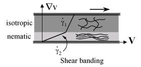
Figure 23 : Schematic representation of the shear banding for system undergoing a shearinduced isotropic-to-nematic transition.
