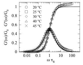
**Figure 8** : Elastic moduli G' and G" as function of the angular frequency for temperatures comprised between 20 °C and 45 °C. G' and G" are divided by the elastic modulus  $G_0$  and the angular frequency  $\omega$  is normalized by the relaxation time  $\tau_R$  of the fluid. Data are for the CPCl-NaSal wormlike micelles in water (0.5 M NaCl) at c = 12 wt. % [123]. The solid lines correspond to the Maxwellian viscoelastic behavior (Eq. 9).
