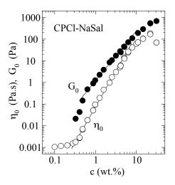
**Figure 9** : Concentration dependences of the static viscosity  $\eta_0$  and of the elastic modulus  $G_0$  obtained for the CPCI-NaSal system. In the semidilute regime (c\* ~ 0.3 wt. %), both quantities exhibit scaling laws as function of the concentration [143]. The exponents are here 2.2 and 3.3, in good agreement with the predictions (see Table II).
