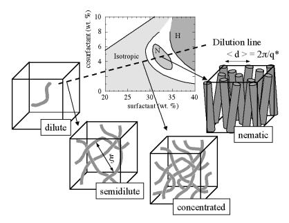
Figure 10 : Schematic illustrations of the different phases encountered in wormlike micellar solutions, from dilute solutions to concentrated mesophases. The phase diagram shown is that of CPCl-Hex (Fig. 6a). <d> denotes the average distance between colinear micelles in the concentrated isotropic and nematic phases.  $\xi$  is the mesh size of the entangled network in the semidilute regime.
