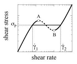
**Figure 22** : Non monotonic constitutive equation assumed for wormlike micelles. The two stable branches at low and high shear rates are separated by an unstable portion [AB]. In the plateau region, the micellar solution demixes in bands of shear rate  $\dot{\gamma}_1$  and  $\dot{\gamma}_2$ .
