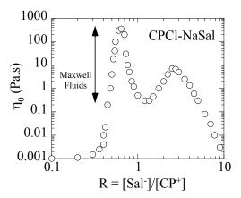
**Figure 7** : Static viscosity  $\eta_0$  for cetylpyridinium chloride–sodium salicylate solutions as function of R (= [Sal<sup>-</sup>]/[CP<sup>+</sup>]). The CPCl concentration is c = 3.6 wt. % (100 mmol). Data are taken from Rehage and Hoffmann [3]. Solutions with viscosity larger than 0.2 Pas are entangled and exhibit a Maxwellian behavior (Eqs. 8 and 9).
