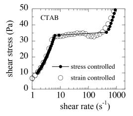
**Figure 13** : Comparison between the steady state shear stress results obtained from controlled strain and controlled stress rheometry in the plateau region. The data are for CTAB-D<sub>2</sub>O wormlike micelles at c = 18 wt. % and T = 32 °C [124]. When stress is applied, the sheared solution jumps from the low shear to the high shear branch of the flow curve. In the lower branch, the stress increases linearly with a static viscosity  $\eta_0 = 6.7$  Pas.
