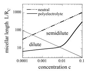
**Figure 1 :** Predictions for the average micellar length of neutral and polyelectrolyte wormlike micelles, as function of the surfactant concentration. The dash-dotted and continuous lines are calculated according to Eqs. 1 and 4 respectively, with parameters taken from [25,26] :  $E = 20 \text{ k}_{\text{B}}T$ ,  $\ell_{\text{B}} R_{\text{C}} v^2 = 1$  and  $n_0 = 1/2$ .
