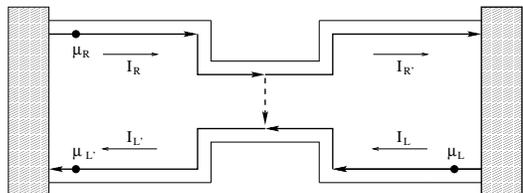
FIG. 3: A schematic illustration of a Hall bar connected to two reservoirs (shaded regions).
