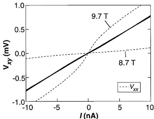
FIG. 1: Plots of the Hall voltage  $V_{xy}$  versus the current  $I$  taken at 0.1-T steps in the  $B$  range from 8.7 T to 9.7 T (the transition from  $1/3$ -QH state to the insulator occurs at  $B_c = 9.1$ ). Dashed traces are of  $V_{xx}$ .  $T = 21$  mK. [Figure taken from Ref. 14].
