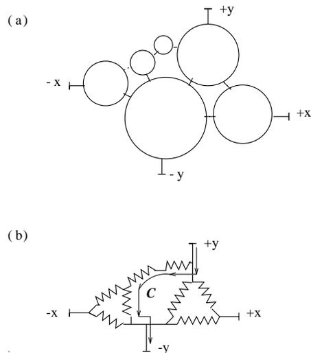
FIG. 4: (a) Typical puddle network, where dotted lines represent constrictions. (b) Corresponding equivalent circuit. Path  $\mathcal{C}$  is denoted by arrows. [Figure taken from Ref. 25].
