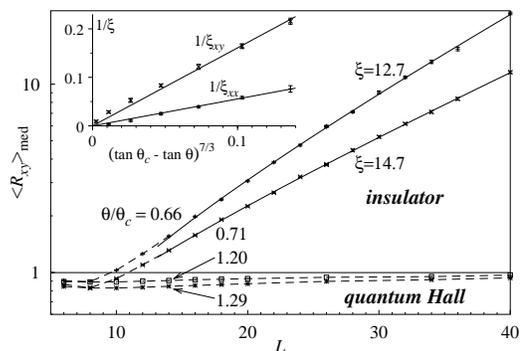
FIG. 5: Finite size scaling of the Hall resistance in the QH and insulator phases.  $\xi$  denotes the localization length, where  $\xi_{xx}$  and  $\xi_{xy}$  correspond to  $\rho_{xx}$  and  $\rho_{xy}$ , respectively. [Figure taken from Ref. 26].
