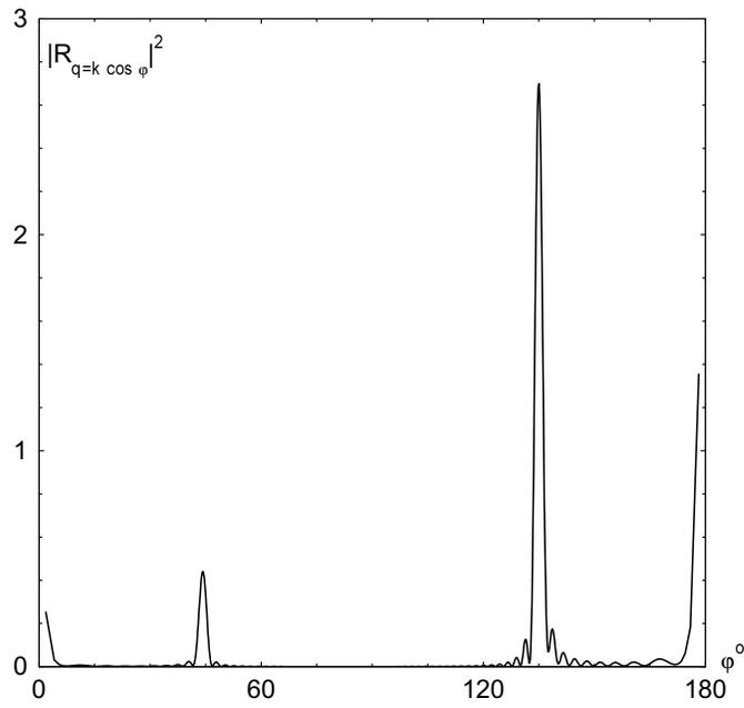
FIG. 2. Angular dependence of the scattering for the case of 2D crystal strip in the spectral region of the exciton resonance. The calculation is performed for the incident wave falling at  $45^\circ$  with respect to the plane of 2D crystal. It is seen that the conventional reflection (maximum at  $135^\circ$ ) is accompanied by the backscattering peaked at  $45^\circ$ .
