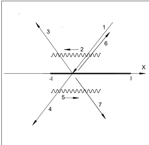
FIG. 1. Scattering of the plane wave by the two-dimensional crystal strip with exciton. 1. – incident plane wave, 2 – exciton produced by the incident wave running from the left to the right and the corresponding polarization. 3,4 – the conventional reflected and transmitted waves, 5 – the wave of polarization related to the exciton reflected from the left edge of the strip. 6,7 – scattered waves produced by the reflected exciton.
