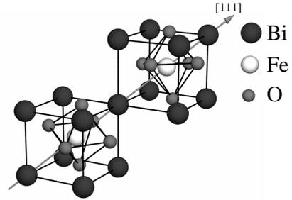
FIG. 1: Schematic view of the  $R3c$  structure built up from two cubic perovskite unit cells. The cations are displaced along the  $[111]$  direction relative to the anions and the oxygen octahedra rotate with alternating sense around the  $[111]$  axis.
