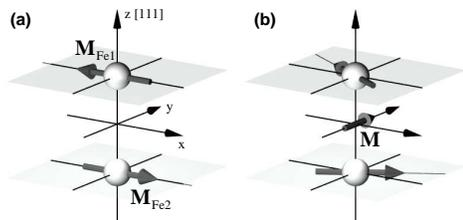
FIG. 2: (a): Starting configuration of our calculation. The magnetic moments,  $\mathbf{M}_{\text{Fe1}}$  and  $\mathbf{M}_{\text{Fe2}}$ , of the two iron atoms in the unit cell are oriented antiferromagnetically and collinearly in the (111) plane, allowing weak ferromagnetism by symmetry. (b): Calculated magnetic structure including the spin-orbit interaction: The two iron magnetic moments rotate in the (111) plane so that there is a resulting spontaneous magnetization,  $\mathbf{M}$ .
