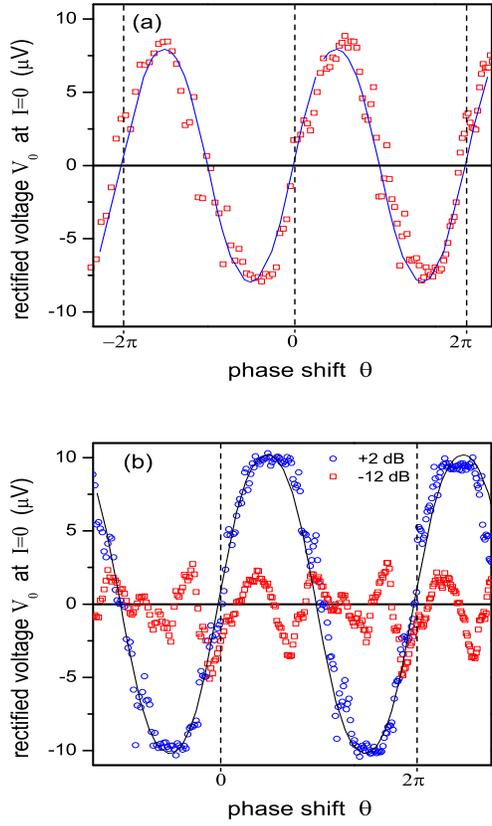
FIG. 3. A dependence of the rectified dc voltage measured at zero dc bias current on the phase shift  $\theta$  between the two harmonics of ac drive. (a)  $f_1 = 1.2$  GHz and  $f_2 = 2.4$  GHz and power  $P_2 = +4$  dB. (b)  $f_1 = 2.4$  GHz and  $f_2 = 4.8$  GHz, for two power levels. Solid lines show results of numerical computation of the voltage for the dimensionless ac bias amplitudes  $E_1 = E_2 = 0.1$  (a) and  $E_1 = E_2 = 0.135$  (b).
