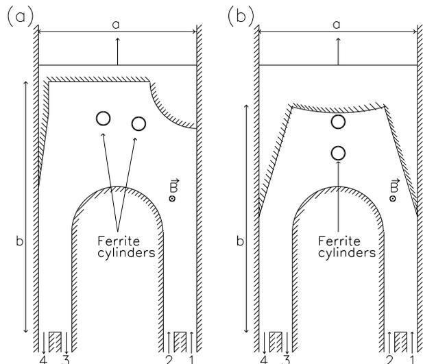
FIG. 1: Sketch of the microwave cavities used in the experiments. (a) The asymmetric cavity has  $a = 237 \text{ mm}$  and  $b$  can vary from 375 to 425 mm. (b) The symmetric one has the same  $a$ , while  $b$  ranges from 340 to 390 mm. The arrows indicate where the ferrite cylinders are placed. The entrance and exit waveguides are denoted by (1,2) and (3,4) respectively.
