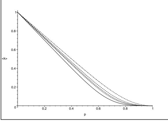
FIG. 6: Plots of  $\langle k \rangle$ , as a function of  $p \in [0, 1]$ , for infinite-length, finite-width strips of the honeycomb lattice. The dashed and solid curves refer to free and periodic transverse boundary conditions, respectively. For a given  $p$ , the dashed curves are, in order of descending value of  $\langle k \rangle$ , for  $2_F \leq (L_y)_F \leq 5_F$ , and the solid curve is for  $4_P$ .
