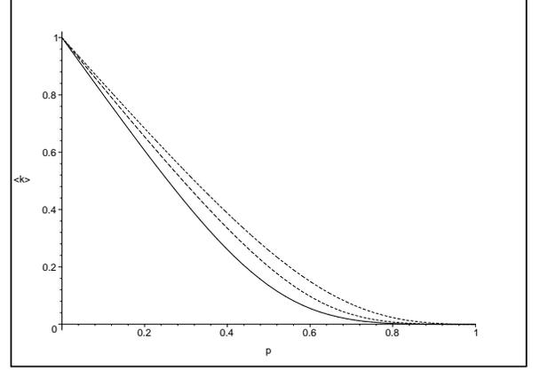
FIG. 7: Plots of  $\langle k \rangle$ , as a function of  $p \in [0, 1]$ , for infinite-length, finite-width strips of the kagomé lattice. The dashed and solid curves refer to free and periodic transverse boundary conditions, respectively. For a given  $p$ , the dashed curves are, in order of descending value of  $\langle k \rangle$ , for  $2_F \leq (L_y)_F \leq 3_F$ , and the solid curve is for  $2_P$ .
