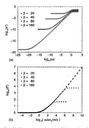
**Fig. 3:** Computer simulations of the random barrier model in three dimensions with the uniform barrier distributions [10]. (a) shows the real part of the conductivity as function of angular frequency (in suitable units [10]) at different inverse temperatures  $\beta$ , (b) shows how these data may be scaled to one single master curve.
