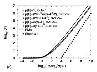
**Fig. 4:** Computer simulations of the random barrier model for several barrier distributions [10]. The figure shows the ac conductivity relative to the dc conductivity as function of scaled frequency at low temperatures. The dots are shown as a guide to the eye giving a line of slope one, while the full line is the classical effective medium approximation (EMA). Today more advanced analytical approximations are available [10].
