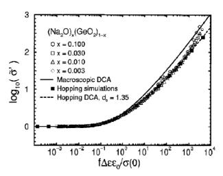
**Fig. 5:** *RBM-prediction for the ac conductivity versus data on Sodium Germanate glasses [21] with varying Sodium concentration. The open symbols are the experimental data while the full symbols give the RBM-universality prediction. "Hopping DCA" is the diffusion cluster approximation [10] (the "macroscopic DCA" is the analogue for a macroscopic model [10]).*
