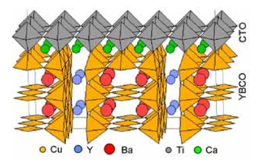
Fig. 1. Schematic crystal structure at the (100) YBCO/CTO interface, showing oxygen coordination of Cu and Ti atoms. O atoms are present at the vertices of each polyhedron. Note the 5-fold coordination of chain Cu at the interface instead of 4-fold in the bulk, and alignment of TiO<sub>3</sub> octahedron along the truncated CuO<sub>2</sub> plane edges.
