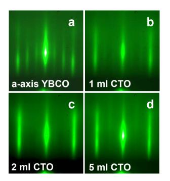
Fig. 2. RHEED images during trilayer deposition. (a) After 2000 Å YBCO; one-third order spots are due to the self-assembled *c*-axis structure lying in the plane of the film. The *a*-axis films are *b*-*c* twinned, with domain sizes ~100 nm inferred from linewidths of diffraction maxima. (b)-(d) Diffraction during barrier growth.
