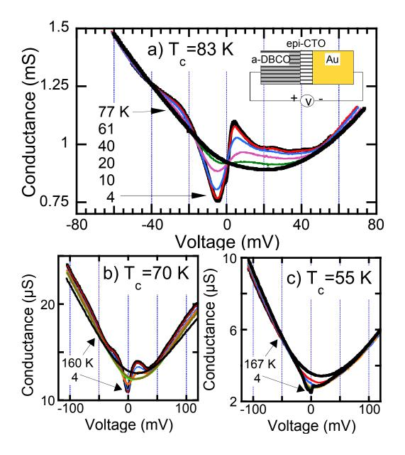
Fig. 3(a-c). Raw conductance data for 3 NIS junctions with different underdopings, showing temperature evolution of the gap structure for occupied state DoS and filling-in of empty state DoS for  $T < T_c$ . P-h asymmetry is strongest at highest  $T_c$ .
