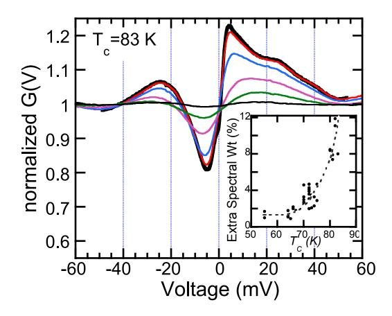
Fig. 4. Normalized G(V) data for junction of Fig. 3(a). Inset shows extra spectral weight at T = 4K in empty state DoS versus  $T_c$  for all junctions (filled state DoS is conserved). Extra spectral weight decreases with decreasing  $T_c$ , disappearing as  $T_c \rightarrow 50$ K.
