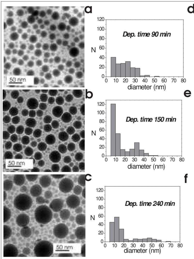
FIG. 4: In (a), (b) and (c) are shown TEM images in plan view of gallium nano-islands self-assembled on Si(100) at surfaces at different deposition times, 90, 150 and 240 minutes respectively. In (d), (e) and (f) histograms of the number of nanoparticles  $N$  versus the diameter  $d$  in nm.
