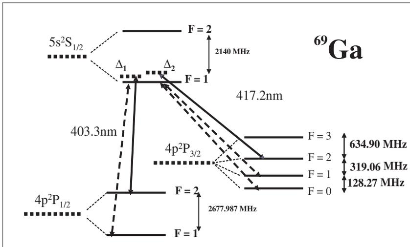
FIG . 2: Hyperfine splittings for the  $^{69}\text{Ga}$  isotope and a choice of fluorescence cycles for laser cooling and repumping. To close the cooling transitions from the ground states (P states) we need blue radiation at  $403\text{ nm}$  and  $417\text{ nm}$  .
