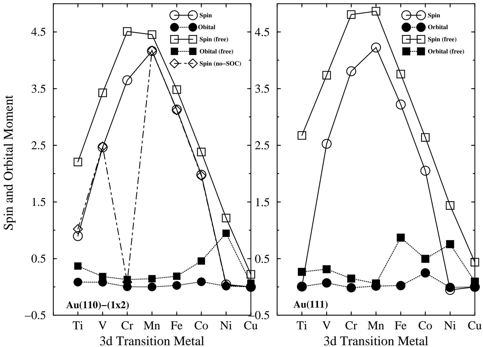
Fig. 2. The spin (solid lines) and orbital (dot lines) moments of the adsorbed 3d atoms and the free standing 3d atoms. The left panel shows the results for Au(110)-(1x2) surface, the right panel for the Au(111) surface. The dot-dash line shows the collinear result for Au(110)-(1x2) surface.
