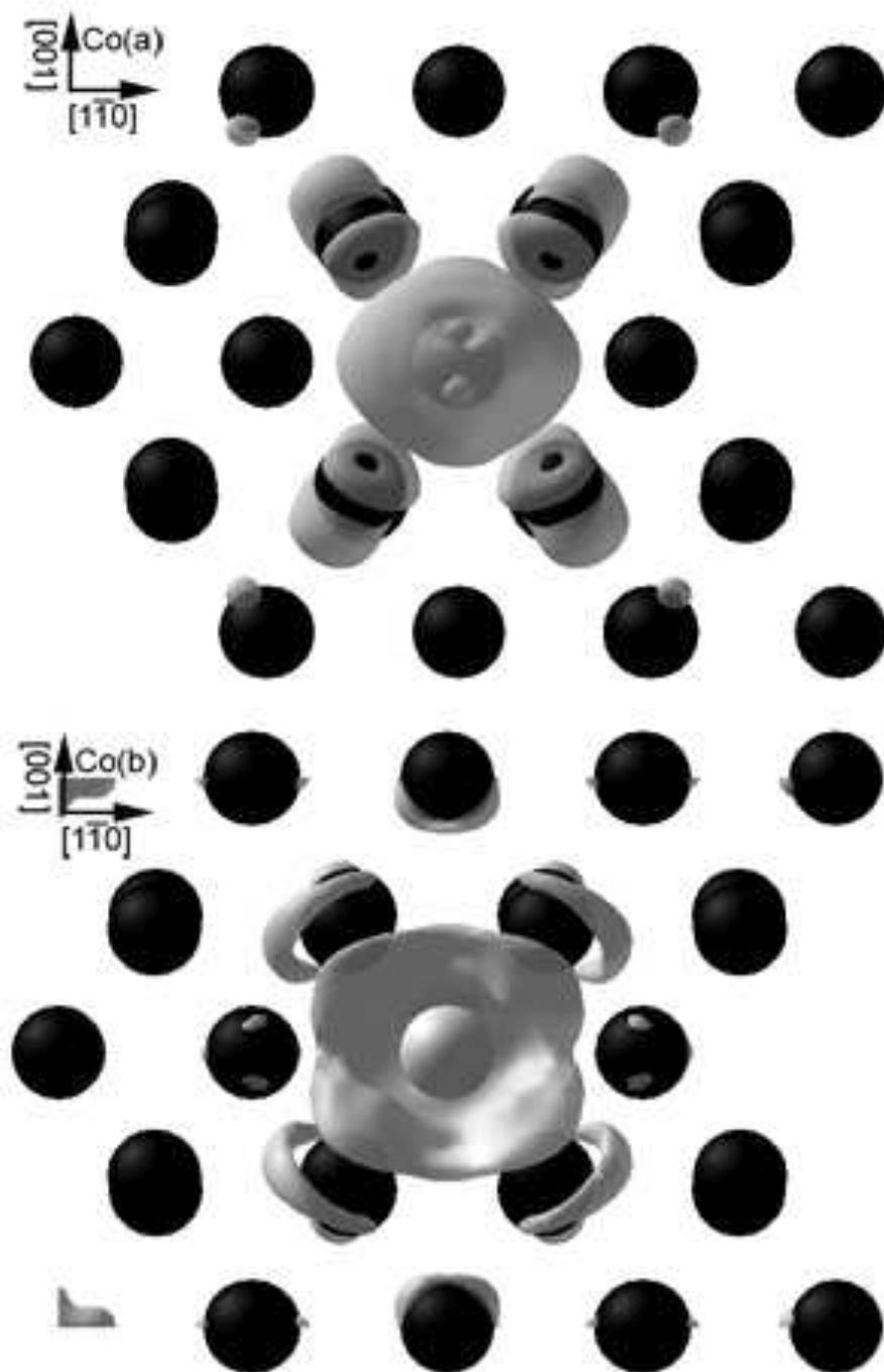
Fig. 5. The magnetic density of the absorbed Co atom which is the components along the quantization axis  $[110]$  and perpendicular to the surface. The magnetic density is defined as  $\rho(\mathbf{r}) = \chi(\mathbf{r}) \cdot \hat{n}$ ,  $\chi$  is the Pauli Matrix. The figure shows the component along the quantization axis. The contour values are  $0.002/\text{\AA}^3$  for the left panel and  $-0.002/\text{\AA}^3$  for the right panel.
