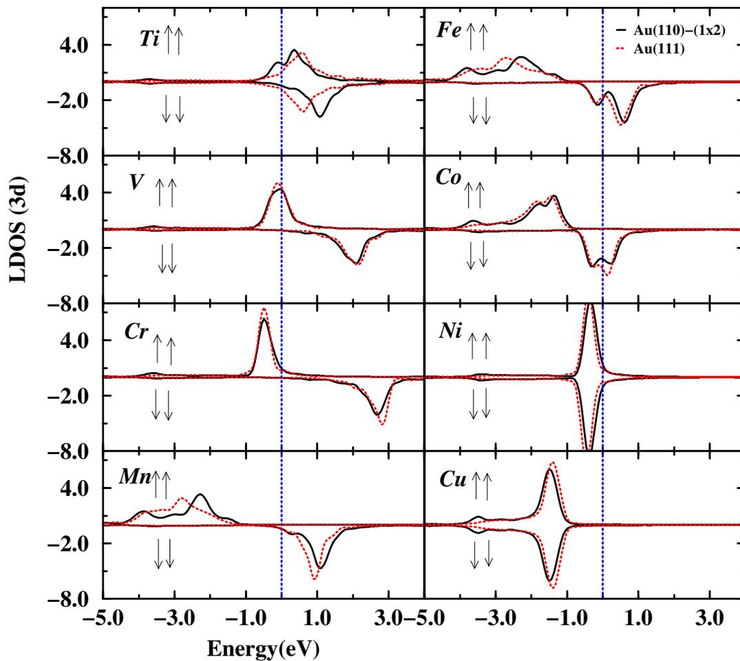
Fig. 4. The 3d densities of state (DOS) for the 3d atoms adsorbed on Au(110)-(1x2) (solid lines) and Au(111) (dot lines) surface.
