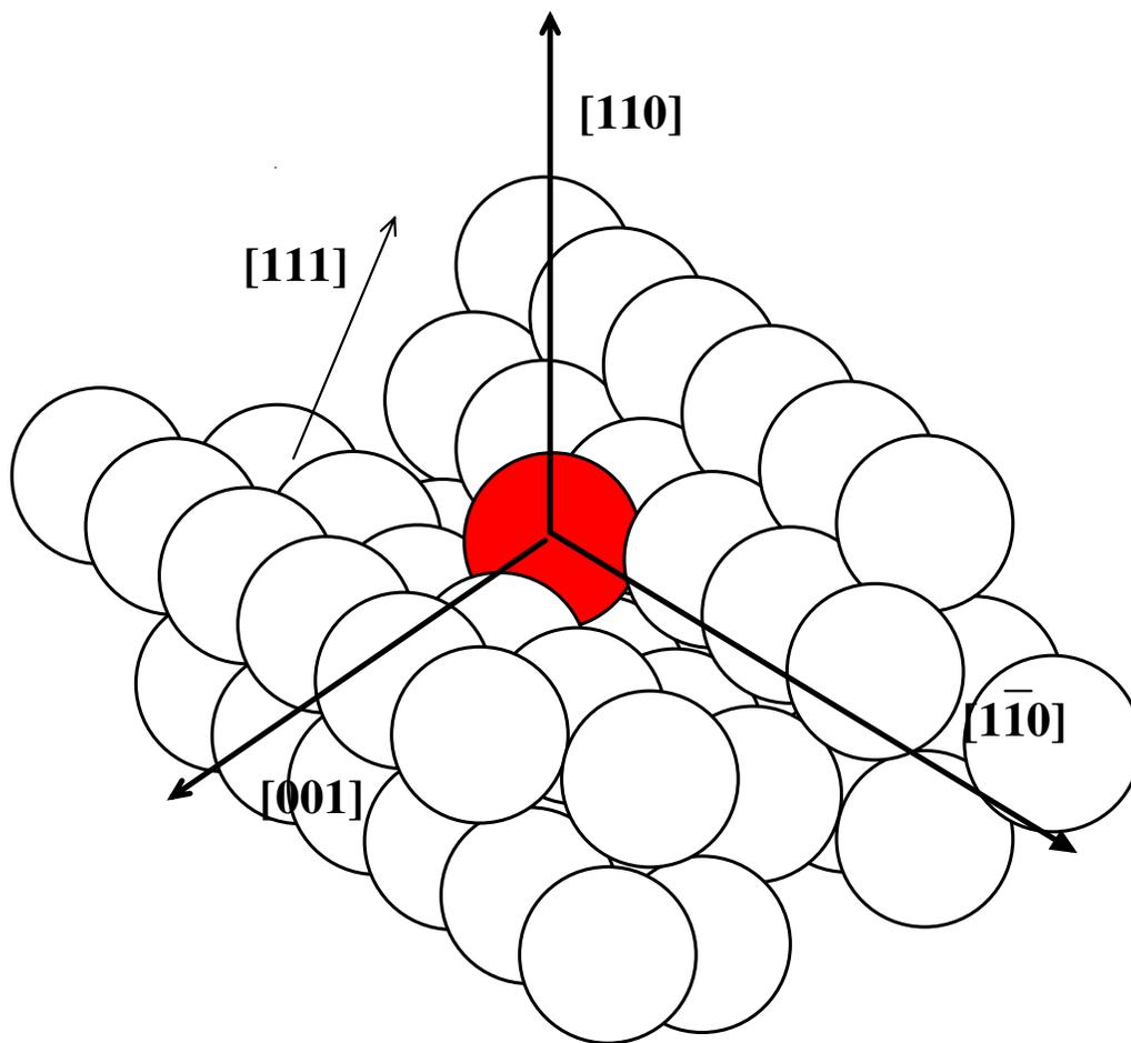
Fig. 1. The schematic diagram of a 3d transition metal atom adsorbed on the Au(110)-(1x2) surface. The trough is along the [110] direction. The normal of the facet of the trough is the [111] direction. The adatom adsorbs on an hollow site in the trough. The white spheres are the Au atoms of the surface, the gray sphere the adsorbed adatom.
