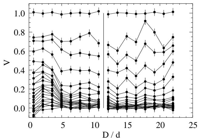
FIG. 7: Scaled velocity,  $V$ , versus distance sheared,  $D$ . The vertical line represents the time at which the system was stopped and restarted in the same direction. There is no significant change in the velocities of the individual slats as a result of the stopping and restarting.
