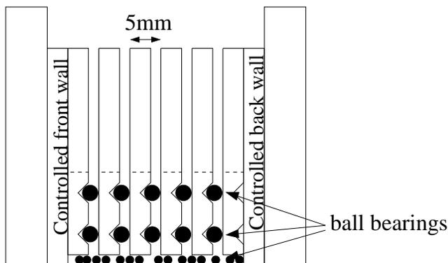
FIG. 3: End View diagram of the parallel plate shear cell. Neighboring slats are separated by two rows of  $\frac{1}{8}$  inch ball bearings. Smaller ball bearings separate all slats from the bottom floor. The front and back walls are moved into and out of the page in order to apply the shear. All other slats are independently movable, and respond to the motion of the grains by moving in the direction perpendicular to the page.
