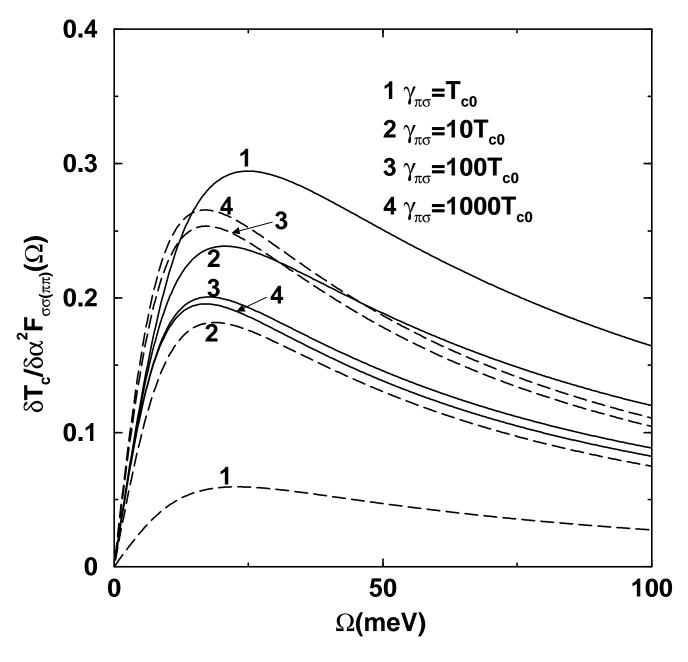
**Figure 2.** The band-diagonal functional derivatives  $\delta T_c/\delta\alpha^2 F_{\sigma\sigma}$  (solid lines) and  $\delta T_c/\delta\alpha^2 F_{\pi\pi}$  (long dashed lines) for four different values of  $\gamma_{\pi\sigma}$  given in units of  $T_{c0}$ .
