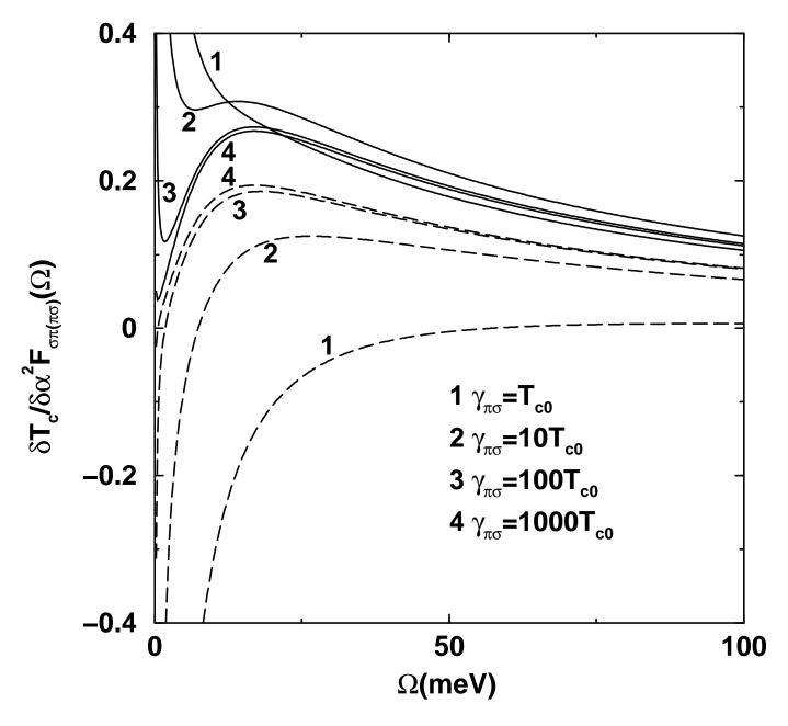
**Figure 3.** The band-off-diagonal functional derivatives  $\delta T_c/\delta\alpha^2 F_{\pi\sigma}$  (solid lines) and  $\delta T_c/\delta\alpha^2 F_{\sigma\pi}$  (long dashed lines) for four different values of  $\gamma_{\pi\sigma}$  given in units of  $T_{c0}$ .
