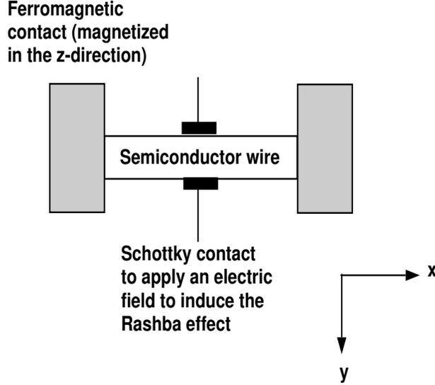
Fig. 1. Physical structure of the magnetic field sensor.
