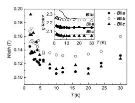
Fig. 3. Temperature dependences of line width and *g*-factor for the various orientations of magnetic field. The solid lines at inset are g(T) data for the pure CuGeO<sub>3</sub> from [10].
