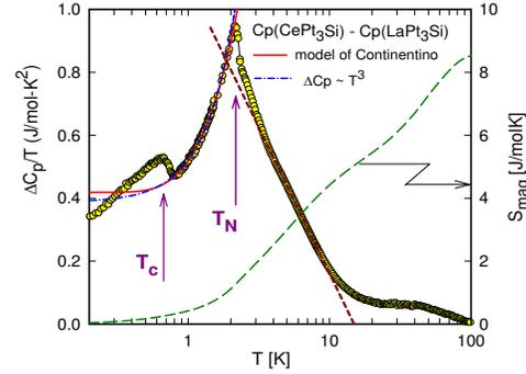
Fig. 1. Temperature dependent magnetic contribution to the specific heat,  $C_p$  of  $\text{CePt}_3\text{Si}$  plotted as  $C_p = T$  on a logarithmic temperature scale. The long-dashed line represents the magnetic entropy (right axis). The short-dashed line is a guide to the eyes and roughly indicates the non-Fermi liquid behaviour. The solid line is a fit according to Eq. 1 and the dashed-dotted line is a fit according to  $C_p = T^3$ .
