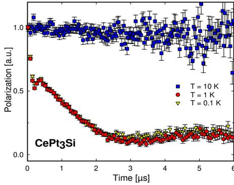
Fig. 4. Zero field depolarisation rate of  $\text{CePt}_3\text{Si}$  at various temperatures.
