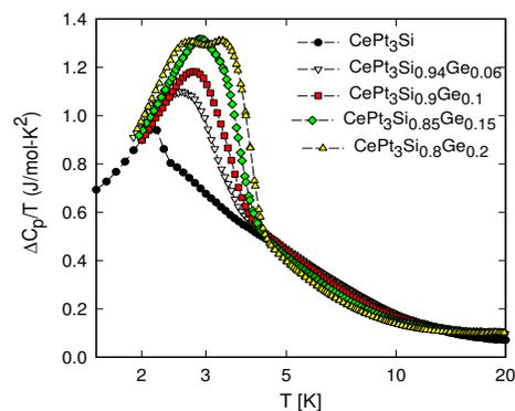
Fig. 8. Magnetic contribution to the specific heat  $C_p$  plotted as  $C_p = T \Delta C_p$  vs.  $T$  for various alloys of  $\text{CePt}_3\text{Si}_{1-x}\text{Ge}_x$ .
