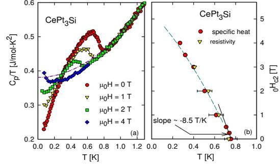
Fig. 3. (a): Temperature dependent specific heat  $C_p/T$  of  $\text{CePt}_3\text{Si}$  for various values of applied fields; the dashed line is a  $T^3$  extrapolation of  $C_p(T)$  at 0 T. (b): Temperature dependence of the upper critical field  $H_{c2}$ . The solid straight line yields  $H_{c2}^0 = 8.5T/K$ ; the dashed line is a guide to the eyes.
