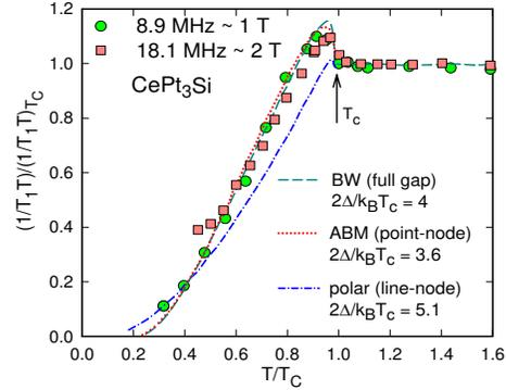
Fig. 5. A plot of  $(1=T_1 T)/(1=T_1 T)_{T_c}$  vs.  $T=T_c$  at 8.9 MHz ( $H = 1 \text{ T}$ ) and 18.1 MHz ( $H = 2 \text{ T}$ ). The dashed line is for the Balian-Werthamer model (BW isotropic triplet SC state) with a value of  $2 = k_B T_c = 4$ . The dotted line assumes a point-node model with  $2 = k_B T_c = 3.6$  and the dashed-dotted line represents a fit by a line-node gap model with  $2 = k_B T_c = 5.1$ .
