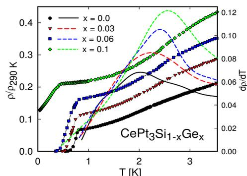
Fig. 7. Low temperature electrical resistivity for various concentrations  $x$  of  $\text{CePt}_3\text{Si}_{1-x}\text{Ge}_x$  (symbols), and temperature derivative  $d\rho/dT$  (lines, right axis).
