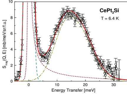
Fig. 2. Magnetic scattering obtained at 6.4 K with the incident energy of 35 meV. The dashed line is for the elastic component with FWHM = 2.4 meV while the short-dashed line represents the quasi-elastic component with FWHM = 0.8 meV. The dashed-dotted line is for the sum of two Lorentzian components centered at 13 and 20 meV with FWHM = 10.0 meV.
