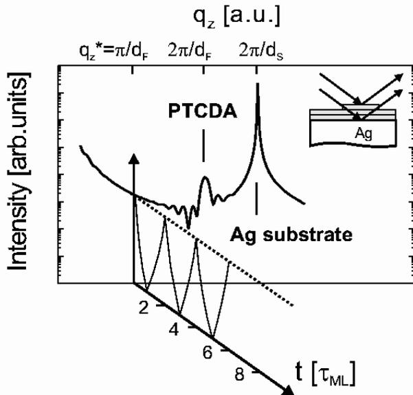
FIG. 2: Simulation of the specular rod of a thin PTCDA film on Ag(111). At the anti-Bragg point of the PTCDA film ( $q_z^* = \pi/d_F$ ), the scattering of subsequent layers interferes destructively (see inset). For layer-by-layer growth, the intensity at the anti-Bragg point oscillates as a function of the deposition time.
