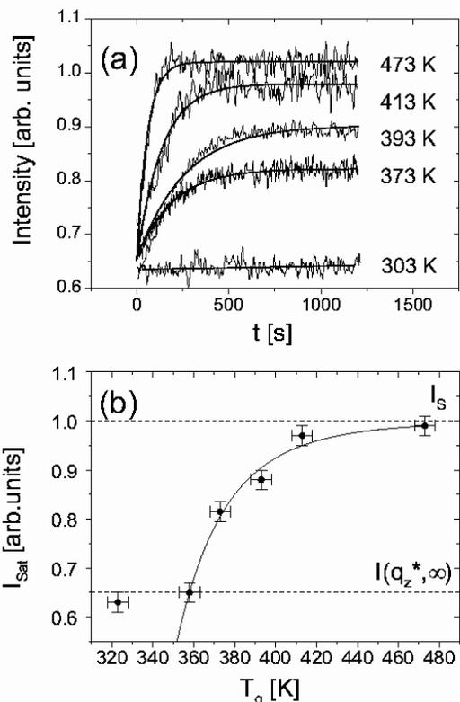
FIG. 4: (a) Intensity at the anti-Bragg point after the deposition of a film as a function of  $T$ , measured for several samples with  $d \approx 50$  Å and  $F = 0.8 - 2$  Å/min. The shutter of the evaporation cell has been closed at  $t = 0$ . (b) Saturation intensity as a function of  $T$ .
