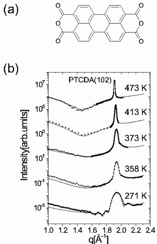
FIG. 1: (a) 3,4,9,10-perylenetetracarboxylic dianhydride (PTCDA). (b) Measured (circles) and calculated (lines) specular rod intensity as a function of the growth temperature  $T$  for samples with  $F = 0.8 - 2$  Å/min and  $d = 50$  Å.
