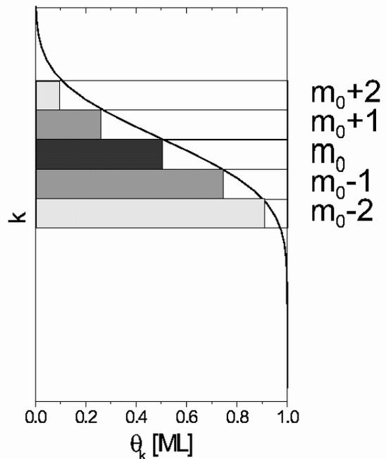
FIG. 7: Schematic explaining the asymptotic intensity. The roughness of the surface is assumed to be Gaussian. The average sample surface corresponds to the layer  $m_0$ . Partially filled layers  $k$  in the same gray scale add up to a completely filled monolayer.
