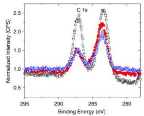
Fig. 3. XPS spectrum showing the binding energy peaks for the C 1s orbitals in the  $Mn_{12}$ -acetate starting material and two ablated films (one created at 8 Hz, 0.8 mJ, and the other at 20 Hz, 2.0 mJ), normalized to 1 at the highest binding energy. See Fig. 1 for key to symbols.
