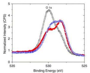
Fig. 2. XPS spectrum showing the binding energy peaks for the O 1s orbitals in the  $Mn_{12}$ -acetate starting material and two ablated films (one created at 8 Hz, 0.8 mJ, and the other at 20 Hz, 2.0 mJ), normalized to 1 at the highest binding energy. See Fig. 1 for key to symbols.
