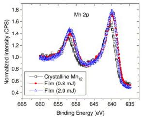
Fig. 1. XPS spectrum showing the binding energy peaks for the Mn 2p orbitals in the  $Mn_{12}$ -acetate starting material and two ablated films (one created at 8 Hz, 0.8 mJ, and the other at 20 Hz, 2.0 mJ), normalized to 1 at the highest binding energy.
