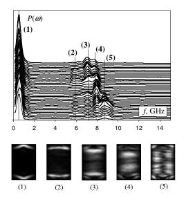
Fig. 3. Oscillation power spectra of a 400 x 500 x 20 nm Py rectangle for wave vectors with  $q_x = 0$  and various  $q_y$  (upper part) in the in-plane field  $H_{\text{ext}} = 600$  Oe along the long side (0y-axis) with maps (below) of the spatial distribution of the  $m_x$  oscillation power for eigenmodes marked with vertical lines on the spectral graph.
