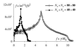
Fig. 1. Power spectrum of  $m_x$ -oscillations for various discretizations. Cusps are the manifestations of the magnon DoS singularity (Fig. 2). The dashed rectangle represents the spectrum expected in the limit of very fine discretization for a low frequency region available for the 40 x 40 discretization.
