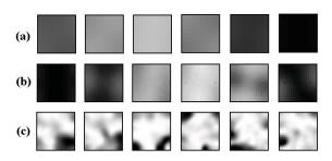
Fig. 7. Typical magnetization patterns (gray-scale maps of  $m_x$ -projections are shown) during the steady-state precession for elements with the sides b = 16 nm(a), 32 nm (b) and 64 nm (c). Non-homogeneous magnetization pattern for the 32 nm element and chaotic domains for b = 64 nm are clearly visible.
