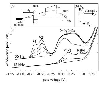
FIG. 1. (a) Conduction band profile of the heterostructure for two different biases, (b) directions of the current and magnetic field, where *x*-*y* is the sample plane. (c) Low-temperature (T = 4.2 K) CV traces for sample B ( $d_1 = 42.5$  nm) taken at low and high frequency. The curves show the influence of an in-plane magnetic field on the s-states (0 T, 3 T, 4 T, 5 T and 8 T, top to bottom) and on the p-states (0 T (dashed), 2 T, 5 T and 8 T).
