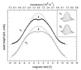
FIG. 2. Tunneling probabilities for the first  $(s_1)$  and second  $(s_2)$  electron in InAs quantum dots (sample A) in <u>k</u>-space, where  $s_2$  is offset for clarity. Filled squares indicate measured data for  $s_1$  and empty squares data for  $s_2$ , the lines are Gaussian fits. The corresponding CV data was measured at 5.1 kHz. The inset shows the full rotational plots of the measured probability densities.
