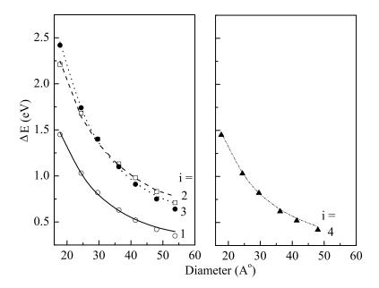
FIG. 5: The variation in E with respect to diameter, d, of the particle for dierent transitions in elective bond order model for CdSe and CdS. The curve through the points are to  $E = A_i = d^{x_i}$ .
