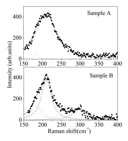
FIG. 7: Ram an spectra for Sam ple A and Sam ple B are shown by led circles. Phonon con nem ent components and surface phonon components are given by dashed and dotted lines, respectively. Solid lines correspond to the best to the experimental data using combined Ram an line shapes
