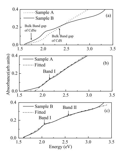
FIG. 4: (a) Optical absorption spectra for Sample A and B. The dotted line is the spectrum for CdSe particles and solid line is for CdSe-CdS core-shell particles. The bulk band gap positions for CdS and CdSe are shown by arrows. (b) and (c) The dashed dotted lines are the nonlinear least square to the experimental curves (solid lines) using elective bond order model.
