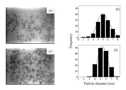
FIG. 2: Low magnication micrographs and histogram of the nanocrystals. (a) is the TEM micrograph and (b) is the corresponding histogram for Samples A. Similarly, (c) is the micrograph and (d) is the corresponding histogram for Sample B.
