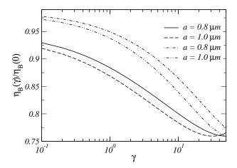
**Figure 2.** Comparison of the normalized Brownian viscosity in the ideal (dash-dotted lines) and non-ideal cases (dashed and solid lines) as a function of the shear rate  $\gamma$  for two values of a. In the non-ideal case, we have chosen  $\Delta_{\gamma} = 0.5$  and  $\delta_{\gamma} = \frac{1}{3}$  which correspond to a density of particles of 0.46, [18].
