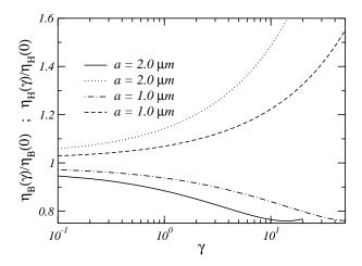
Figure 1. The Brownian (solid and dashed-dotted lines) and hydrodynamic (dashed and dotted lines) viscosities as a functions of the shear rate for different values of the radius of the Brownian particle. This figure shows the shear thinning and thickening effects. The values of the parameters we have used are  $\beta_0 \simeq 10^6 s^{-1}$ ,  $D_0 \simeq 10^{-6} cm^2 s^{-1}$  and  $\rho \simeq 0.2 cm^3$ .
