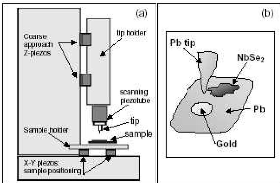
FIG. 1: Scheme of the STM unit (a) and its composite sample holder (b) used in the low temperature laboratory of the Universidad Autónoma de Madrid.
