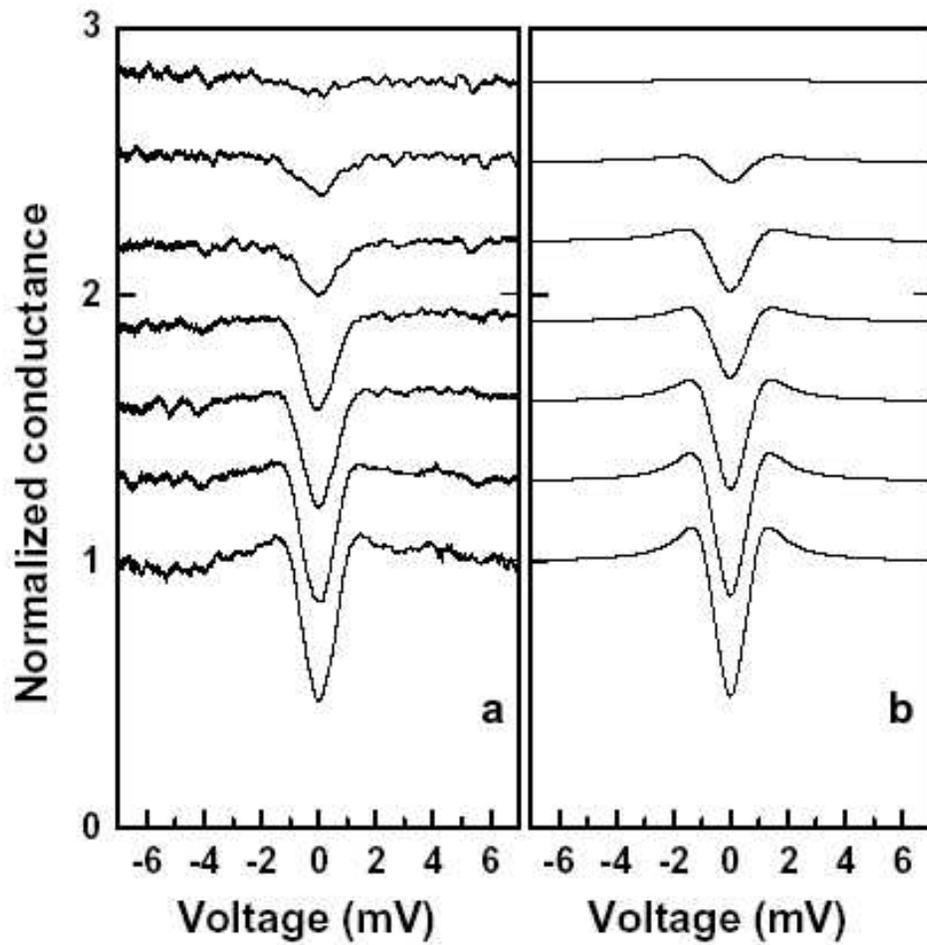
FIG . 15: After the creation of the nanostructure, if the tip is transported to a region of the sample which is at, curves characteristic of N-S junctions are obtained, with the superconducting density of states showing a large amount of low energy excitations (experiment, a), explained within the variable geometry model of Ref.[116] (calculated curves in b). From bottom to top,  $T = 1.0; 1.5; 2.0; 2.5; 3.0; 3.5; 4.0$  K
