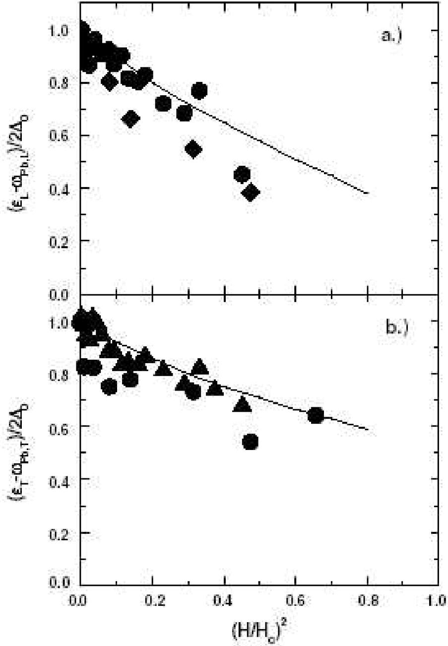
FIG. 14: The strong coupling features corresponding to the longitudinal (a) and transversal (b) phonon modes ( $\epsilon_{L,T}$ ) is shown as a function of the magnetic field. The data are extracted directly from the position of the corresponding features in the tunneling density of states ( $\epsilon_{L,T}$ ), and plotted normalized to the superconducting gap at each field. The theory developed by [143] (lines) explains the data. From [140].
