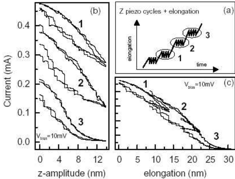
FIG . 4: (a) Schem atic indication of the tim e evolution of the process of elongation of the nanobridge. (b) I-z curves as recorded in a real nanobridge fabrication. Each group of curves (1,2 and 3) correspond to a di erent stage of the elongation of the nanobridge, i.e., a di erent neck. These curves can be arranged in order to account for the total elongation of the nanobridge (c). (Data from [64])
