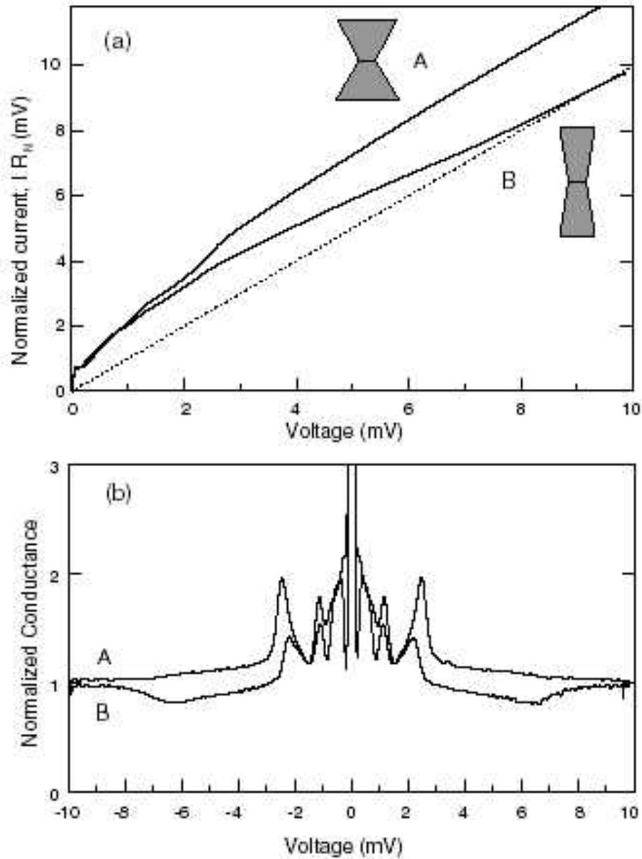
FIG. 9: Normalized  $I-V$  (a), and conductance (b) curves corresponding to two different nanobridges with the same nominal resistance, 500  $\Omega$ . Clear heating effects appear for the long and narrow bridge (B). The geometries of both nanobridges are sketched. The dotted curve in (a) indicates the normal state situation. (Data from Ref.[64], see also [46])
