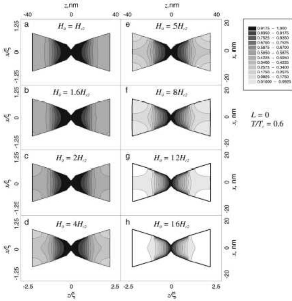
FIG. 12: Distribution of the superconducting order parameter in a nanostructure at different magnetic fields (at  $T/T_c = 0.6$ ) (from [138]). Superconductivity survives at the central part of the neck up to fields much higher than the bulk critical one.
