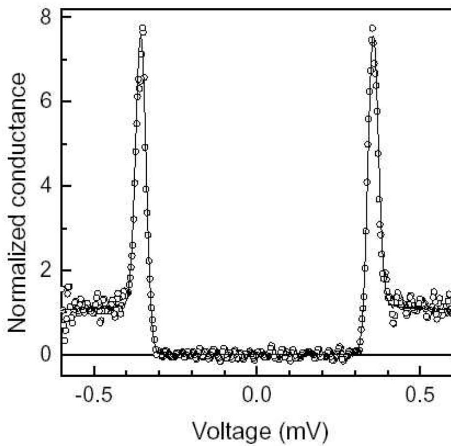
FIG. 6: A  $1\text{-Al}$  tunnelling conductance curve obtained at 70 mK and its corresponding fitting. Data taken from [92].
