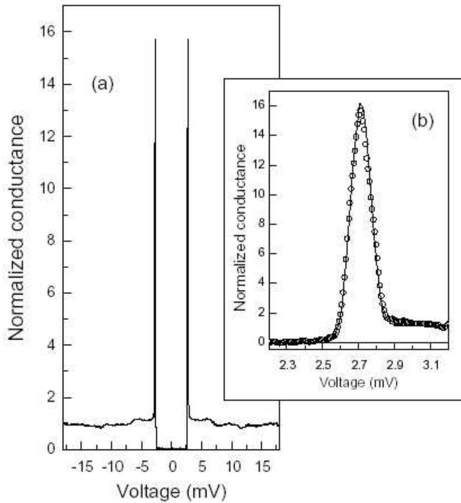
FIG. 7: (a) Tunnelling conductance curve obtained in a  $^3\text{He}$  cryostat at 0.3K with tip and sample of Pb ( $R_N = 1\text{M}\Omega$ ). (b) Zoom of the gap edge. The theoretical conductance (line) has been calculated with the parameters described in the text, in order to reproduce the experimental curve (circles). Data taken from [92].
