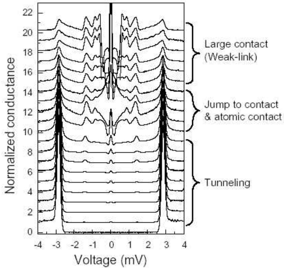
FIG. 5: Evolution of the conduction spectra along the different stages of the creation of a Pb nanostructure (nanobridge). For a given nanostructure, it covers resistances from  $100 \Omega$  (large point contact) up to  $10 M\Omega$  (vacuum tunneling). Atomic contact takes place for resistances about  $10 k\Omega$ . Measurement performed at  $1.8 K$ . Data from Ref. [64].
