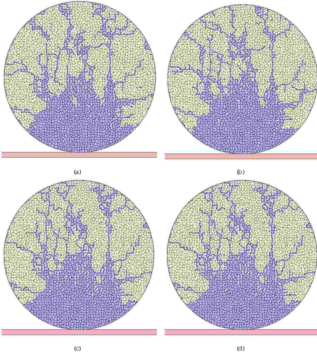
FIG. 3: The reassembled snapshots of normal and oblique impacts at different velocities keeping the normal component constant as 500cm/sec. The crack patterns are almost same in all cases. (a)  $\theta = 90^\circ$ . (b)  $\theta = 75^\circ$ . (c)  $\theta = 60^\circ$ . (d)  $\theta = 45^\circ$ .
