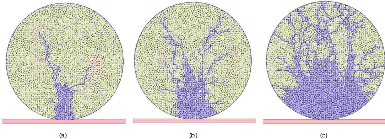
FIG. 2: Final reassembled states of the break-up process of a disc of radius 30 cm at different impact velocities dropped on a hard frictionless plate. (a)  $v_0 = 100$  cm/sec. The cone is not fully developed and only few oblique cracks are present. (b)  $v_0 = 200$  cm/sec. More oblique cracks develop and travel a greater distance. (c)  $v_0 = 600$  cm/sec. Both oblique cracks and secondary cracks are present.
