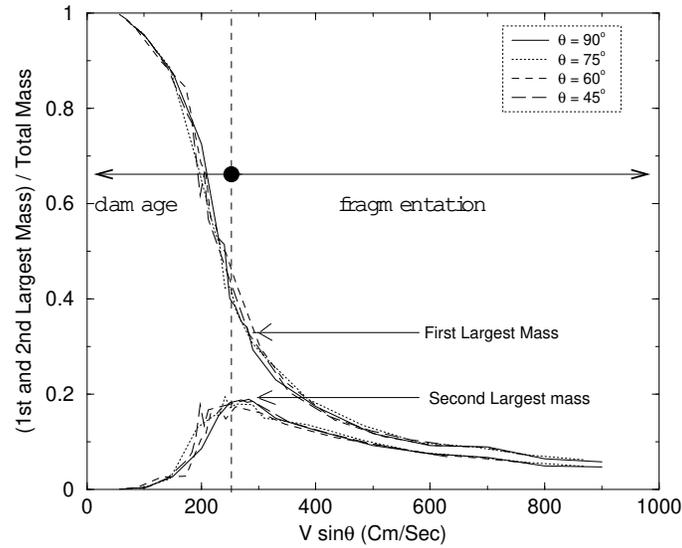
FIG .4: The mass of the first and second largest fragment as a function of the normal component of the impact velocity  $v_0 \sin \theta$  at different impact angles and velocities  $v_0$  for a system size 30 cm . The vertical dashed line indicates the critical point, furthermore, the damaged and fragmented regions are also shown .
