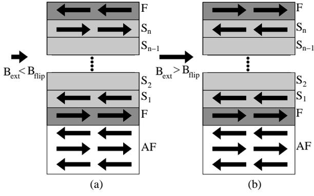
FIG. 1: Schematic of the ferromagnet magnetizations and the magnetic fields felt by the superconducting layers for (a)  $\mathcal{B}_{\text{ext}} < \mathcal{B}_{\text{flip}}$  and (b)  $\mathcal{B}_{\text{ext}} > \mathcal{B}_{\text{flip}}$ .
