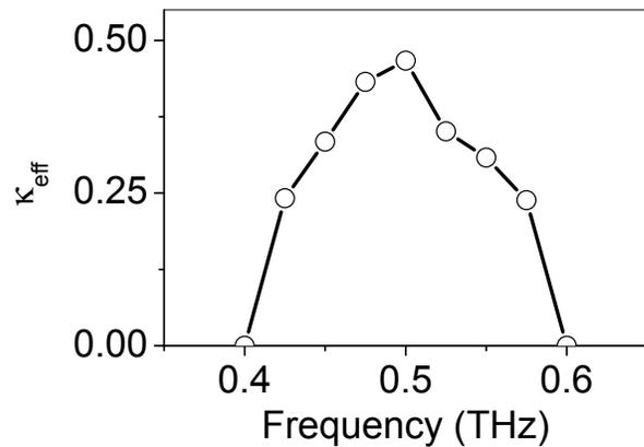
FIG. 6: effective extinction coefficient of Si photonic crystals.
