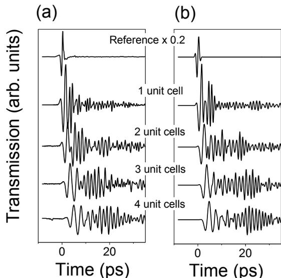
FIG. 3: Terahertz pulses transmitted through photonic crystals with different thickness. The thickness is indicated in the figure as the number of unit cells (1 unit cell =  $276\mu\text{m}$ ). Measurements are plotted in (a), while the corresponding FDTD simulations are displayed in (b). For clarity a vertical offset has been introduced to the different pulses. The uppermost pulses are the reference, i.e., the instrumental response of our setup.
