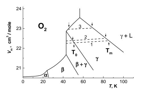
Fig.1. V-T phase diagram of solid  $O_2$  plotted using data of [1,2]: (----) - molar volumes; arrows show the onset of single-phase region and melting.
