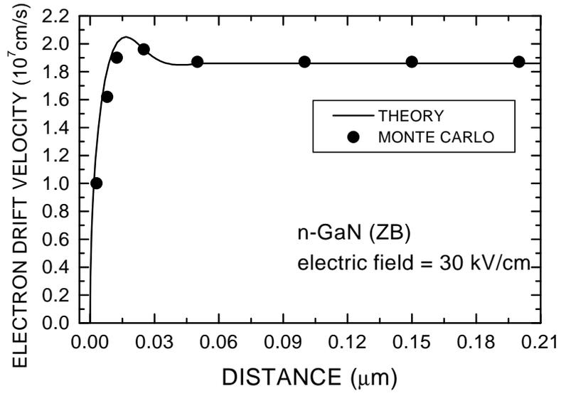
FIG. 4: Evolution of the electron-drift velocity in  $n$ -GaN in terms of the travelled distance, comparing the results of the NESEF-based kinetic theory with a Monte Carlo simulation (Full circles from Ref.[20]): zincblende  $n$ -GaN for an electric field intensity 30kV/cm and  $T_0 = 300K$ .
