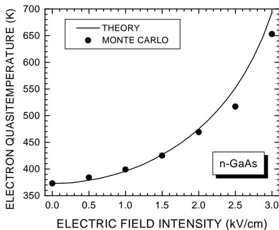
FIG. 1: The electron quasitemperature *vs.* the electric field intensity, in the steady state of *n*-GaAs, comparing the results of the NESEF-based kinetic theory with a Monte Carlo simulation (full circles from ref.[15]).
