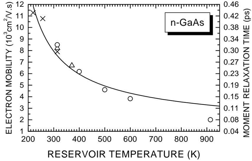
FIG. 2: Electron mobility (and momentum relaxation time) in  $n$ -GaAs for different values of the reservoir temperature, comparing the results of the NESEF-based kinetic theory with experimental data (up triangle from Ref.[14],  $\times$  from Ref.[17], empty circles from Ref.[18]).
