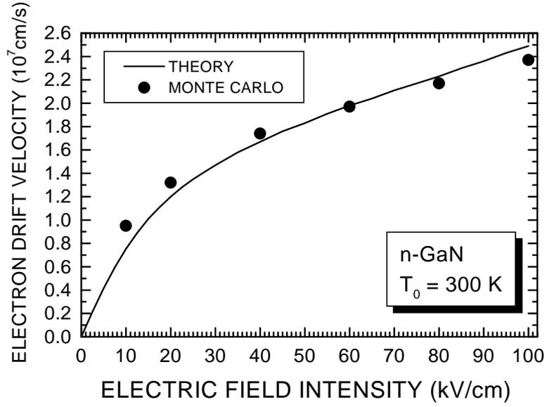
FIG. 3: Electron-drift velocity *vs.* electric field intensity in *n*-GaN, comparing the results of the NESEF-based kinetic theory with a Monte Carlo simulation (Full circle from Ref.[19]), with  $T_0 = 300K$ .
