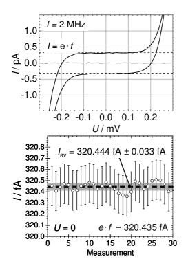
Fig. 3: I-V curves with current plateaus at I = ef (top panel, f = 2 MHz) and precision measurement of the zero-bias current (bottom panel). Each data point was derived from a measurement averaging over two minutes, including current reversal. The grey bar shows the (expanded) uncertainty for the mean value  $I_{av}$ .
