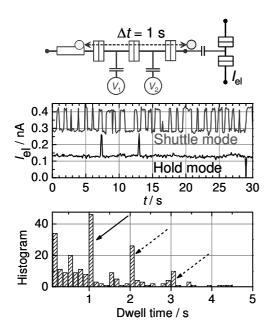
Fig. 5: Time series traces of the electrometer signal in the hold and the shuttle-pumping mode  $(\pm e, wait time 1 s)$ in type A sample (middle panel, traces are offset for clarity). Because of the small total capacitance only island charge states with + e, 0, and - e were possible. The bottom histogram of panel shows а the electrometer signal during shuttlepumping.
