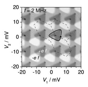
Fig. 2: Plot of the current (grey-scale) delivered by a 3j r-pump pumping at f = 2 MHz while scanning the dc gate voltages  $V_{1,2}$ . Within the dark (light) triangular regions, appearing in the typical "honeycomb" pattern, current is pumped in positive (negative) direction. The circumference of these regions (solid curve) reflects the trajectory of the ac gate signals.
