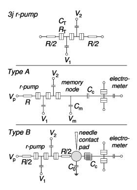
Fig. 1: Circuit schemes of different sample types investigated.
