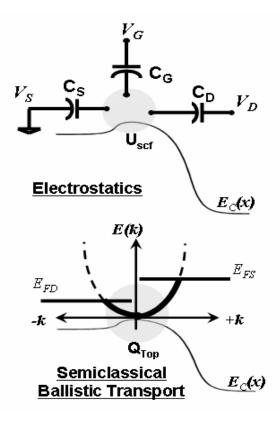
Fig. 4 Illustration of the essential aspects of the semi-numerical ballistic FET model.
