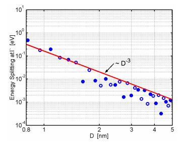
Fig. 3 The splitting energy (at the  $\Gamma$  point) *vs.* wire width (*D*) for the simulated Si nanowires. The closed circles are for the wires with an odd number of atomic layers while the open circles are for the ones with an even number of atomic layers. The splitting energy fluctuates with *D* and the envelope decreases according to  $\sim D^{-3}$ .
