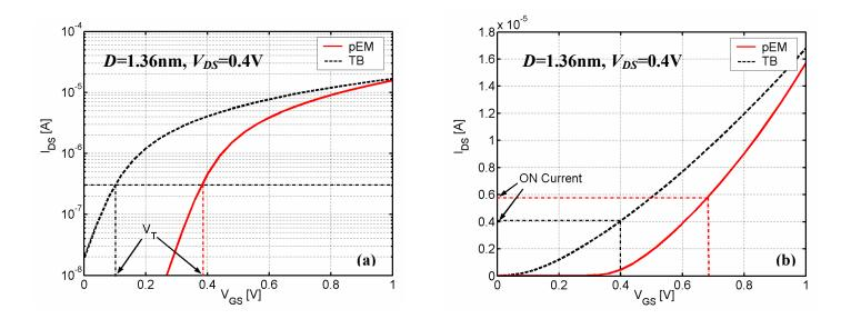
Fig. 5 The  $I_{DS}$  vs.  $V_{GS}$  curves for a square SNWT with D=1.36nm in both (a) a semi-logarithmic scale and (b) a linear scale. The oxide thickness is 1nm, the temperature is 300K, and the drain bias is 0.4V. The dashed lines are for the results based on the tight-binding (TB) *E-k* relations while the solid lines for the parabolic effective-mass (pEM) results.
