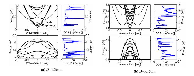
Fig. 2 The tight-binding *E-k* relations and the corresponding density-of-states (DOS) for the simulated Si nanowire structures with (a) D=1.36nm and (b) D=5.15nm. The conduction band for the thinner wire (D=1.36nm) displays significant band splitting at the  $\Gamma$  point.
