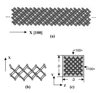
Fig. 1 (a) The atomic structure of a square nanowire (D=1.36nm) with a [100] transport direction. (b) A unit cell of the square nanowire illustrated in (a). (c) The schematic diagram of the cross section of the square nanowire. D demotes the edge length of the square cross section and the four faces of the square are all along the equivalent <100> axes.
