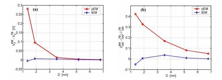
Fig. 7 The wire width dependence (*D*) of the errors,  $V_T^{EM} - V_T^{TB}$  in (a) and  $(I_{ON}^{EM} - I_{ON}^{TB})/I_{ON}^{TB}$  in (b), associated with the effective-mass approximations. The solid lines with circles are for the parabolic effective-mass (pEM) approximation while the dashed lines with diamonds are for the tuned effective-mass (tEM) approach.
