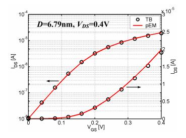
Fig. 6 The  $I_{DS}$  vs.  $V_{GS}$  curves for a square SNWT with D=6.79nm in both a semi-logarithmic scale (left) and a linear scale (right). The oxide thickness is 1nm, the temperature is 300K, and the drain bias is 0.4V. The circles are for the results based on the tight-binding (TB) *E-k* relations while the solid lines for the parabolic effective-mass (pEM) results.
