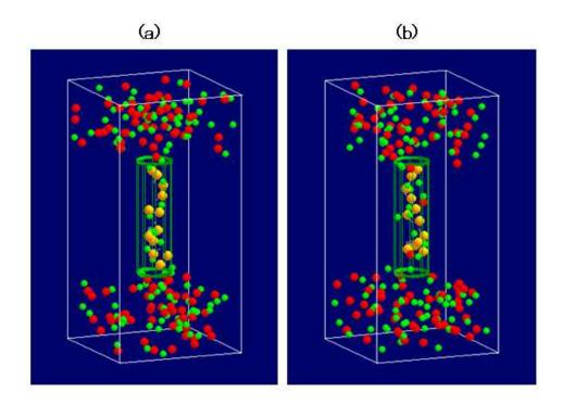
FIG.2: Snapshot of the ion distribution with ssDNA in the pore for  $"_m = 2$  (a) and  $"_m = 80$  (b). G reen and red spheres are counterions and coions, respectively and orange spheres represent the charged phosphate groups of DNA (the neutral sugars and bases are not shown).
