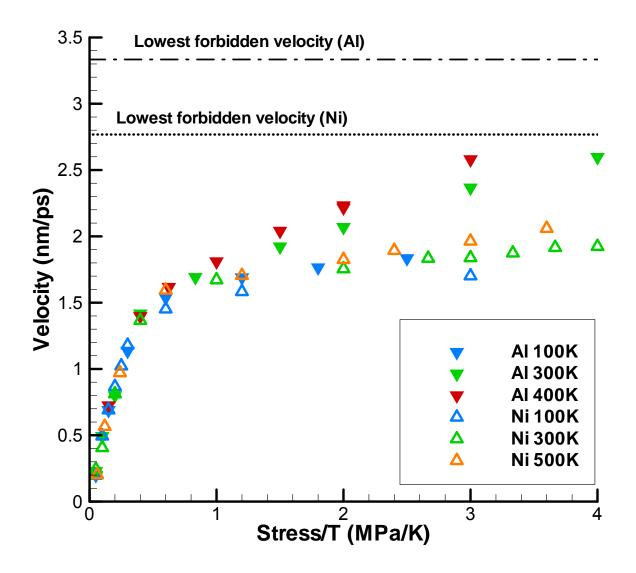
Figure 3. Velocity as a function of the applied shear stress divided by the temperature  $(\sigma/T)$  for screw dislocations in Al and Ni. For  $\sigma/T < 0.4$  MPa/K, the velocity is roughly linear and depends only on  $\sigma/T$ . For  $\sigma/T > 0.6$  MPa/K, the velocity no longer depends solely on  $\sigma/T$ .
