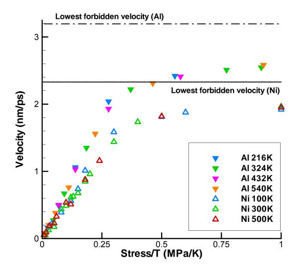
Figure 2. Velocity as a function of the applied shear stress divided by the temperature  $(\sigma/T)$  for edge dislocations in Al and Ni. The velocity is nearly linear for  $\sigma/T < 0.3$  MPa/K, and remains a function of  $\sigma/T$  up to  $\sigma/T = 1.0$  MPa/K, but saturates at a value below the lowest forbidden velocity.
