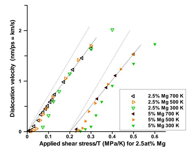
Figure 4. Velocity as a function of the applied shear stress divided by the temperature  $(\sigma/T)$  for edge dislocations in Al-Mg random substitutional alloys (2.5at%Mg and 5.0at%Mg are shown). The data for Al5.0at%Mg is offset by 0.2 MPa/K for clarity. Solid lines: linear fits to 500K data. Dashed lines: fit for pure Al edge data, for reference.
