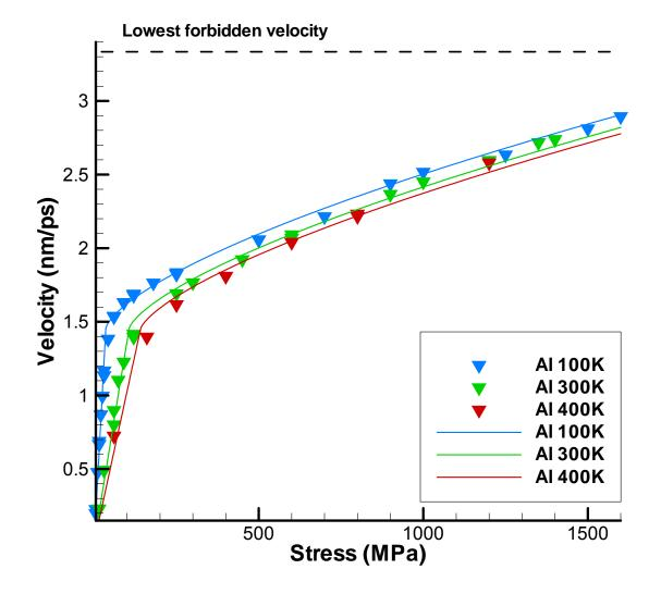
Figure 8. Aluminum screw dislocation velocity as a function of the applied shear stress. The lines are a fit of the data to Eq. (3).
