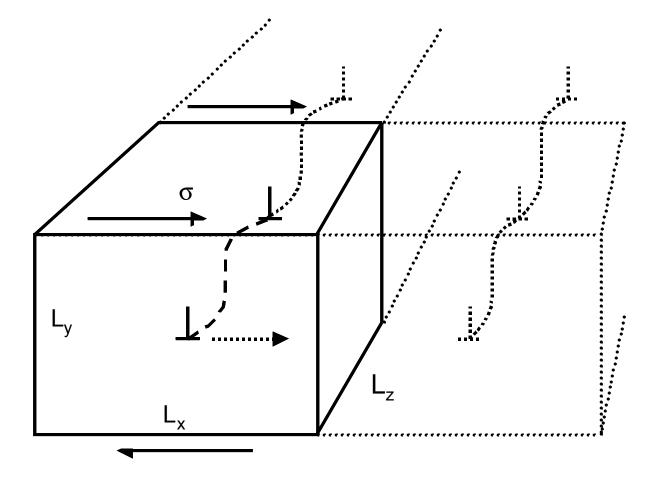
Figure 1. Simulation cell of sides  $L_x,\,L_y,\,L_z$  with single dislocation subject to an applied shear stress  $\sigma$  .
