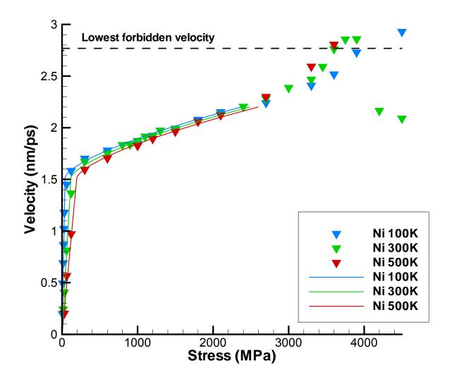
Figure 9. Nickel screw dislocation velocity as a function of the applied shear stress. The lines are a fit of the data to Eq. (3).
