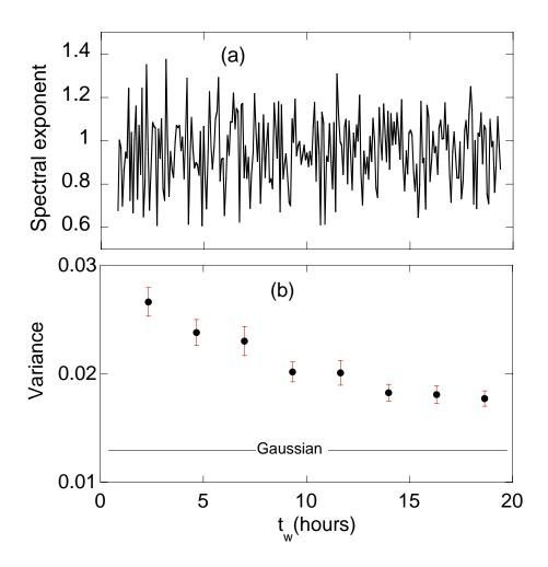
Figure 2. The spectral exponent, measured by a power-law fit between 0.1 Hz and 1 Hz, is plotted (a) vs. waiting time following a quench to 302 K. In (b) the variance of spectral exponent measured over 2.3 hour windows and averaged over 12 quenches is plotted vs. waiting time for 302 K. The prediction for Gaussian noise is shown.
