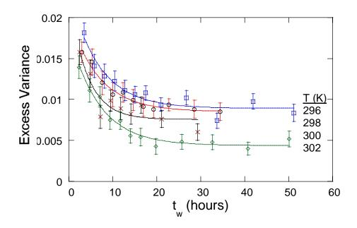
Figure 3. The excess (above Gaussian) variance in spectral exponent (0.1 Hz-1 Hz) is plottted vs. waiting time for several temperatures (indicated). For waiting times < 20 h the data are averaged over 2.3 h windows and 10 to 20 quenches. After 20 h the variances from several adjacent 2.3 h windows are averaged for 3 to 5 quenches.
