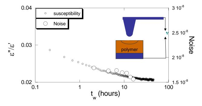
Figure 1. The dielectric susceptibility (ratio of imaginary to real components) measured at 1 Hz in a macroscopic sample is plotted vs. waiting time following a temperature quench from 315 K to 302 K. The polarization noise measured during aging in a nanoscopic sample in a band centered on 1.4 Hz at 302 K is also shown. Inset: noise measurement setup showing SPM tip, sample and probed volume.
