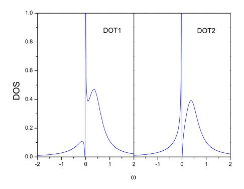
FIG. 5: The local density of state for each quantum dot. Used parameters are  $U = 4.0, \bar{\epsilon} = -2.0, \Delta \epsilon = 1.0, t_c = 1.0.$
