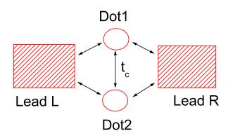
FIG. 1: Parallel double quantum dots with interdot tunneling  $t_c$ .
