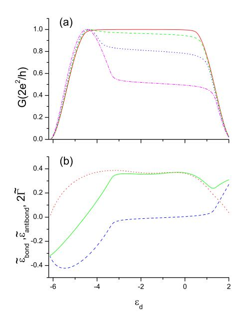
FIG. 3: (a)The linear conductance as a function of the dot level at zero temperature. Used parameters are U = 4.0,  $\Gamma^L = \Gamma^R = 1.0$ , and the interdot tunneling  $t_c = 0.0$ (solid line), 0.2(dashed line), 0.5(dotted line), 1.0(dash-dotted line). (b) The bonding state energy  $\tilde{\epsilon}_{bond}$ (solid line), the antibonding state energy  $\tilde{\epsilon}_{antibond}$ (dashed line) and the level broadening  $2\tilde{\Gamma}$  of the bonding state(dotted line) for  $t_c = 1.0$ .
