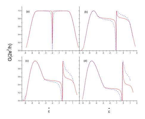
FIG. 4: The linear conductance at zero temperature for parallel double quantum dots with different energy levels. Used parameters are U = 4.0,  $\Gamma^L = \Gamma^R = 1.0$ . The energy level differences are  $\Delta \epsilon = 0.5$  (solid line), 1.0 (dashed line). (a), (b), (c), and (d) correspond to the interdot tunneling  $t_c = 0.0, 0.5, 1.0, 1.5$ , respectively.
