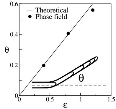
FIG. 2: Kink angle versus surface energy anisotropy predicted as  $\theta = \frac{1}{2}$  and extracted from phase-field simulations (filled circles) for  $G = G_c + 1\%$ . Inset: phase-field simulation for  $\epsilon = 1.2$  ( $\theta = \frac{1}{2}$  contours are equally spaced in time).
