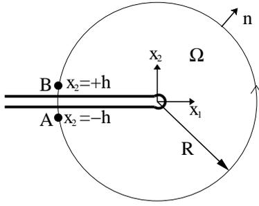
FIG. 1: Spatially discrete crack tip region with  $\Omega = 1/2$  contour separating broken and unbroken material (thick solid line).
