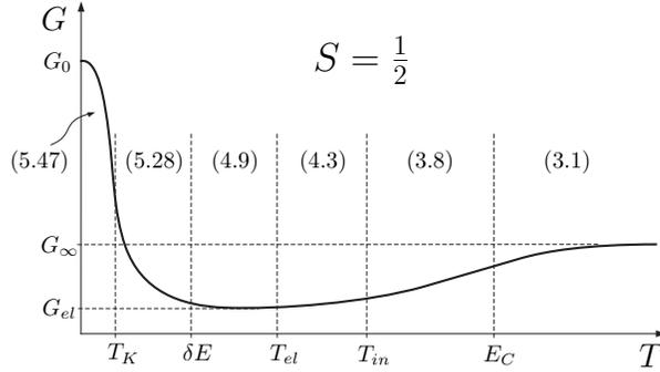
Fig. 3. Sketch of the temperature dependence of the conductance in the middle of the Coulomb blockade valley with  $S = 1/2$  on the dot. The numbers in brackets refer to the corresponding equations in the text.
