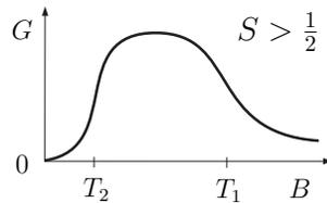
Fig. 6. Sketch of the magnetic field dependence of the Kondo contribution to the linear conductance at zero temperature. The conductance as function of temperature exhibits a similar non-monotonic dependence.
