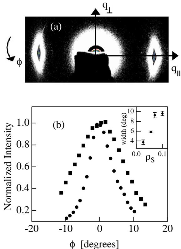
FIG. 7: (a) X-ray intensity distribution from SmA correlations in an anisotropic aerosil gel ( $\rho_S = 0.035 \text{ g cm}^{-3}$ ). The underlying nematic order is long range while the SmA order is short range. (b) The sample mosaic spread for anisotropic gel samples of density  $\rho_S = 0.027 \text{ g cm}^{-3}$  (circles) and  $\rho_S = 0.100 \text{ g cm}^{-3}$  (squares) at 300.1 K. (Reproduced with permission from Liang *et al.*, 2004.)
