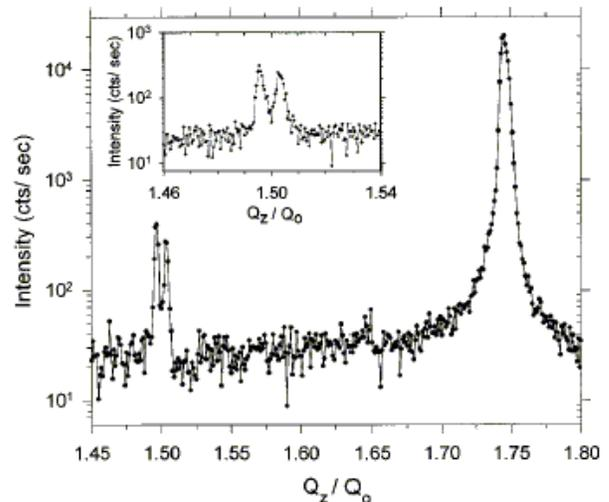
FIG. 4: X-ray intensity versus wave-vector transfer for the  $\text{SmC}_{FI2}^*$  phase of MHDDOPTCOB. (Reproduced with permission from Mach *et al.*, 1999.) The splitting becomes resolvable for the second order peak.
